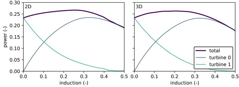
Figure 3: Power production in steady state for varying induction on upstream turbine, in 2D (left) and 3D (right), with turbine configuration as in Figures 1 and 2 respectively. Maximum greedy power production occurs for  $a = 0.33$ . Within this model, lowering the induction on the upstream turbine to  $a = 0.27$  leads to a 3.6% gain in total power.
