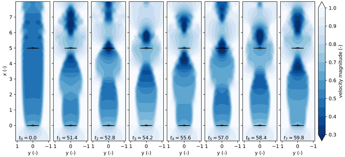
Figure 6: Snapshots of the flow field from the 2D free-vortex wake simulation under uniform inflow in positive  $x$  direction with the induction signal applied to the turbine as shown in Figure 5. The effects of the periodic induction excitation can be seen in the structure of the wake and appear to enhance wake breakdown.
