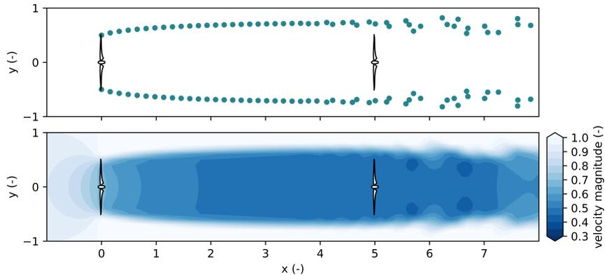
Figure 1: Illustration of the 2D FVW for uniform unit inflow without yaw misalignment and with a constant induction factor  $a = 0.33$ . The pairs of vortex points (top) can be used to calculate the velocity at any point, allowing visualisation of a dense velocity field (bottom). The figure illustrates the two-turbine case where the second turbine performance is calculated from the flow velocity 5 D downstream.
