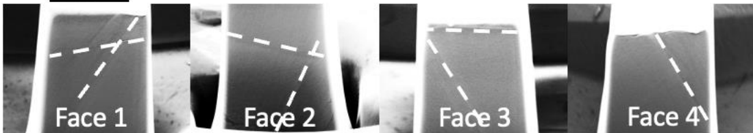
Figure A 2. SEM micrographs of deformed micropillars for pillar 1, pillar 2, pillar 3 and pillar 4 showing all four surfaces with experimental slip traces annotated. The micrographs for pillar 3 and pillar 4 are modified from ref [27].
