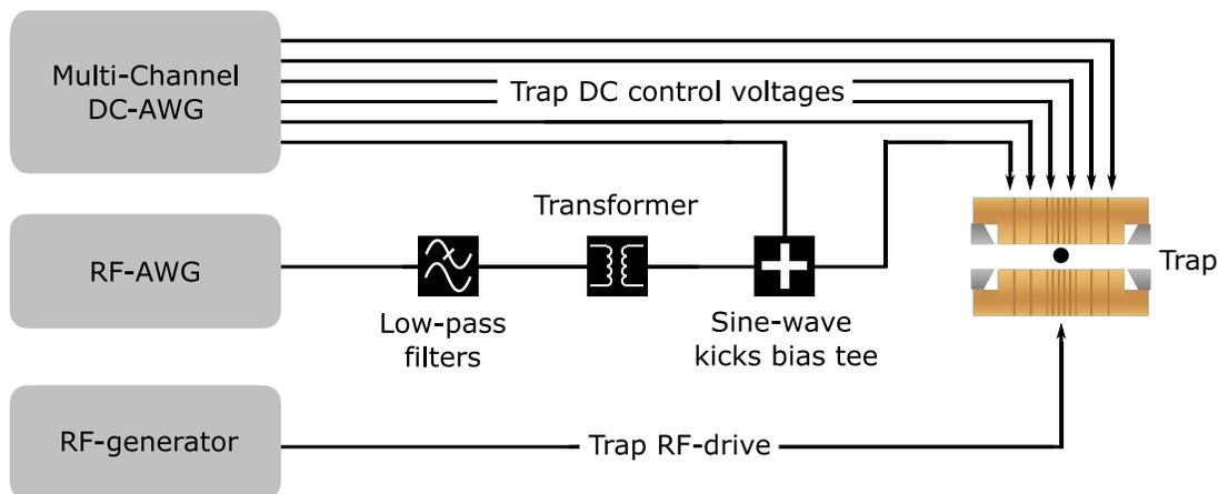
**Figure 3.** Schematic of the electronic setup. For applying fast electric pulses on trapped ions, we used two arbitrary waveform generators (AWGs), low-pass filters for each DC electrodes and a 1:1 ratio transformer for isolating the RF-AWG from noise. Simultaneous application of DC voltages and sinusoidal pulses on one trap electrode elongated along the trap axis was carried out by feeding them through a bias tee.
