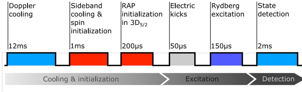
**Figure 5.** Pulse scheme for the experimental sequence labelled with the time duration applied in the experiment. Cooling and state initialization were carried out using the 397 nm (blue) and 729 nm lasers (red). Coherent motional states were generated by applying an electric kick (in grey). Rydberg states were excited in a resonant two-photon process using 213 nm and 287 nm lasers (violet). The final state is detected using fluorescence detection techniques (see also Fig. 2).
