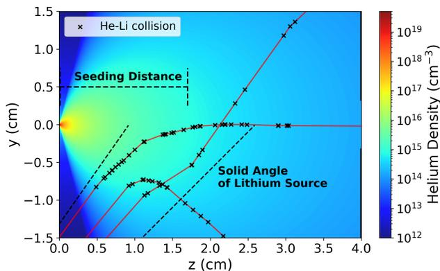
FIG. 2. Example simulation results for 200 sccm of He flow. Trajectories are shown along with the location of collisions denoted with an “x”. Three distinct type of particles are shown: one which is deflected by the jet, one seeded and within the capturable solid angle of the skimmer (half angle of 0.079 radians) and one which undergoes collisions but passes through the jet without fully thermalizing.
