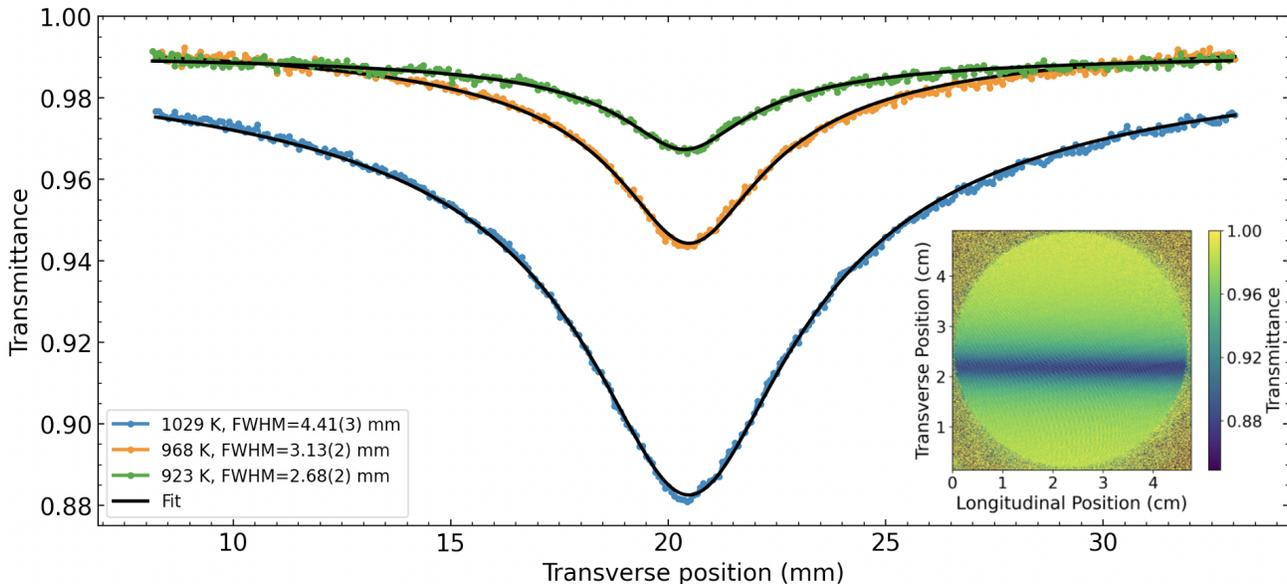
FIG. 11. Absorption spectroscopy results at the atomic focus. The data is fit to the Abel transform of a Lorentzian profile to determine the FWHM of the atomic beam. In the bottom right corner is an example absorption image.
