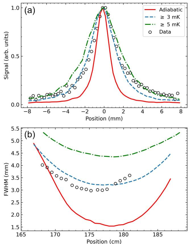
FIG. 14. Simulated focus results versus fluorescence data. (a) Measured transverse profile vs simulated transverse profile. (b) FWHM versus distance from nozzle for data and simulation. In the legend adiabatic refers to a pure adiabatic expansion, while 3 and 5 mK refer to introducing a temperature floor in the expansion.
