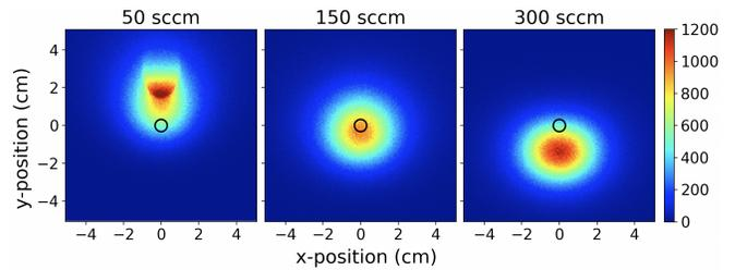
FIG. 13. 2D histogram of  $5 \times 10^6$  simulated particles and the positions of all particles that pass the xy plane 4.1 cm from the nozzle. The seeding distance is 1.7 cm and the black circle indicates particles that are within the capturable solid angle of the skimmer projected to the xy plane. Data is binned into  $0.25 \times 0.25$  mm boxes. The number above each plot gives the helium flow rate.
