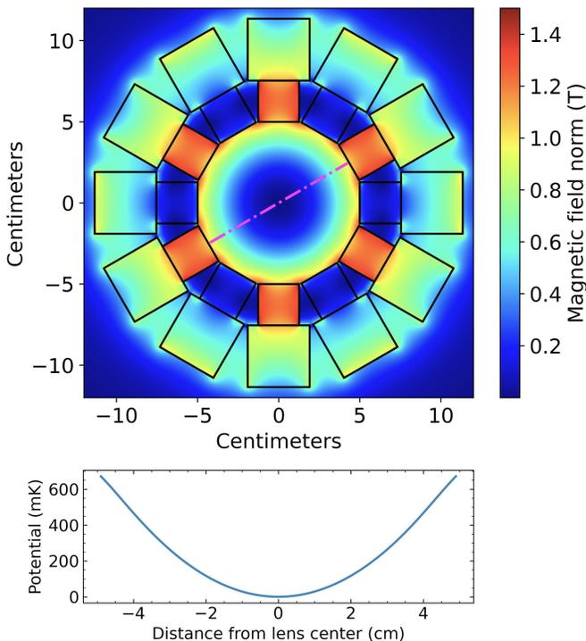
FIG. 5. (a) Simulated norm of the magnetic field at the center-plane of our lens. (b) A lithium atom's magnetic potential as a function of position along the dash-dotted line in (a).
