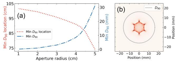
FIG. 6. (a) Size and location of minimum  $D_{90}$  versus aperture of atom lens for point source of particles.  $D_{90}$  is diameter of circle containing 90% of atoms, and location is distance from the end of the atom lens. (b) Heatmap of particle intensity at minimum  $D_{90}$  for full lens aperture. Contrast was increased for readability.
