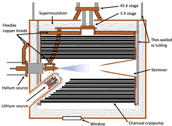
FIG. 3. Schematic of the two stage cryogenic region
