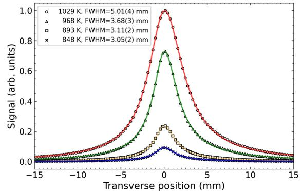
FIG. 10. Spatial profile at the atomic focus for different oven temperatures fit to a q-Gaussian distribution. The data is from fluorescence spectroscopy and is normalized to the peak signal at the highest oven temperature.
