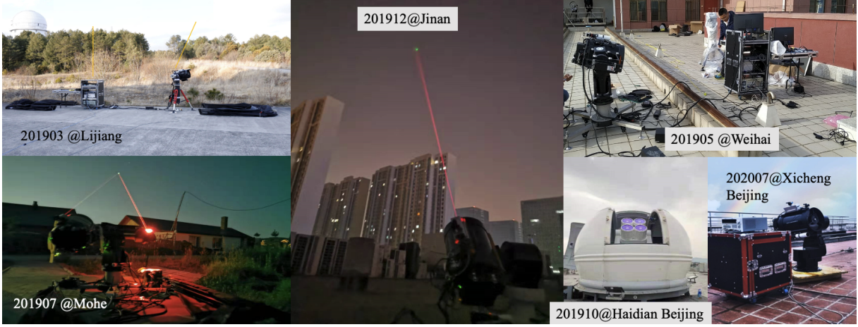
FIG. 45 Experimentally demonstrating the feasibility of satellite-to-ground QKD with compact ground stations. Up to 2020, QKD with Micius satellite and the compact ground station, in many cities of China, such as Beijing, Jinan, Weihai, Lijiang, Mohe, and so on. The typical sifted key rate is \sim 2 kbps.
