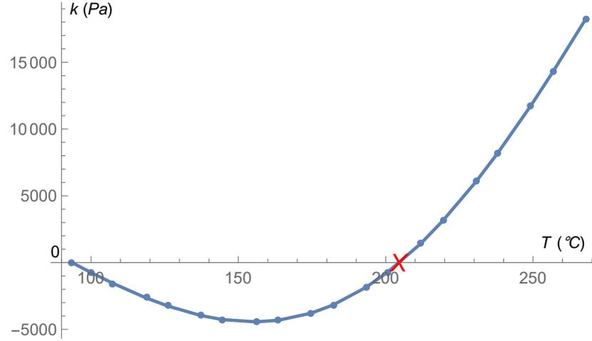
FIG. 5. Graphs associated with the  $k$  in Pa as a function of  $T^{\circ}\text{C}$  in the *second linear approximation* (37). The  $x$  axis is associated with the Celsius temperature and the  $y$  axis with the pressure  $k$  expressed in Pascal. The dots represented  $k$  values calculated with the software *Mathematica*<sup>TM</sup>. In this case, the Leidenfrost temperature highlighted by a red cross is  $T_L \approx 204^{\circ}\text{C}$ .
