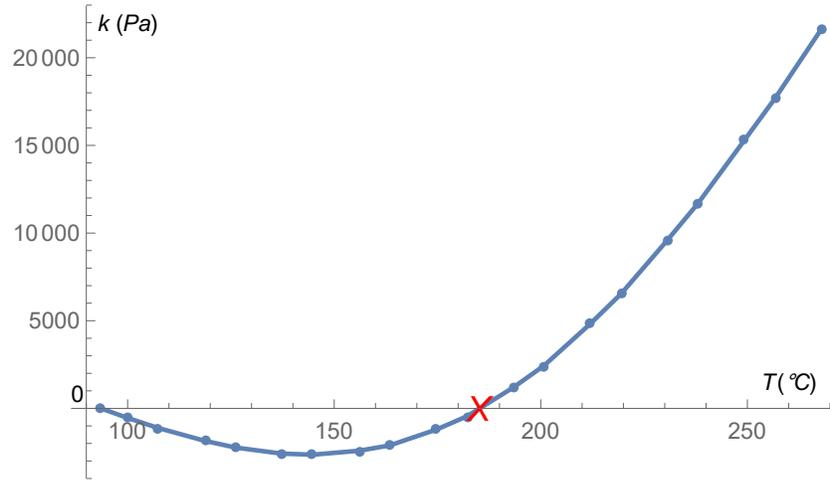
FIG. 4. Graphs associated with the  $k$  in Pa as a function of  $T^{\circ}\text{C}$  in the *first linear approximation* (36). The  $x$  axis is associated with the Celsius temperature and the  $y$  axis with the pressure  $k$  expressed in Pascal. The dots represented  $k$  values calculated with the software *Mathematica*<sup>TM</sup>. In this case, the Leidenfrost temperature highlighted by a red cross is  $T_L \approx 185^{\circ}\text{C}$ .
