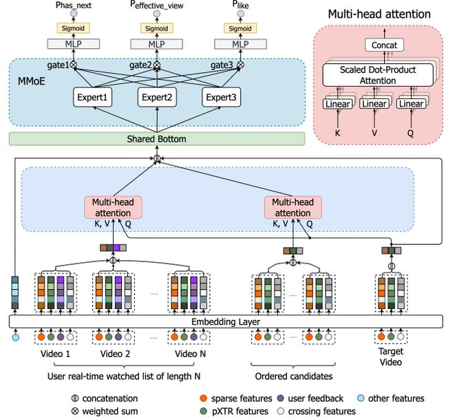
**Figure 3: Architecture of the on-device ranking model.**
