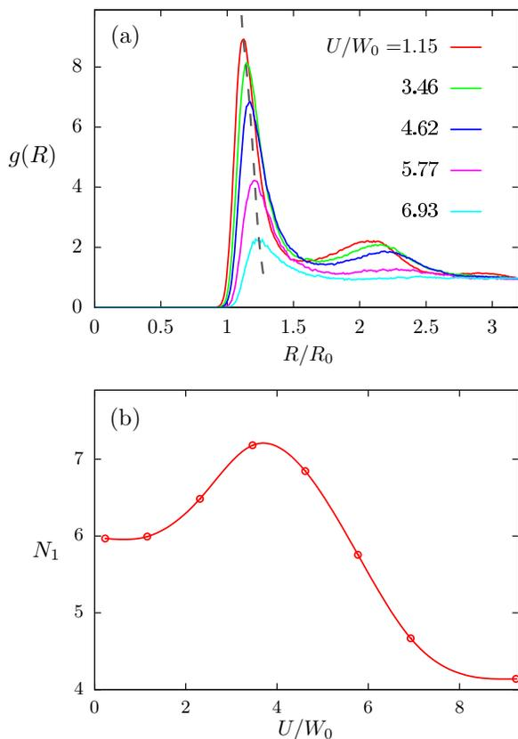
FIG. 6: (a) The pair distribution function  $g(R)$  at different values of Hubbard parameter. The reference length  $R_0$  is given by the equilibrium distance of the binding curve  $E(R) = -2h(R) + \phi(R)$  between a pair of atoms. The Mott transition occurs at  $U_c \sim 7W_0$ . (b) the effective coordination number  $N_1$  versus Hubbard parameter  $U$  obtained from the DMFT-MD simulations.
