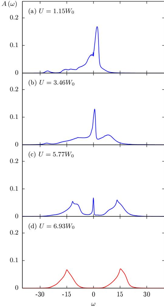
FIG. 2: The spatially and temporally averaged electron spectral function  $A(\omega)$  at varying values of Hubbard parameter obtained from DMFT-MD simulations. The Mott transition occurs at a critical  $U_c \sim 6.9W_0$ . Panel (c) shows a three-peak structure consisting of two Hubbard bands and a sharper quasi-particle peak at the center.
