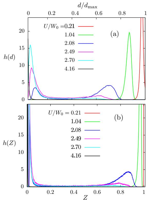
FIG. 12: Histogram of (a) local double occupancy  $d_i$  and (b) quasi-particle weight  $Z_i$  at varying Hubbard repulsion obtained from the DMFT-MD simulations. The Mott transition occurs at a critical  $U_c \sim 3.1W_0$ . The distribution function  $h(d)$  in the intermediate  $U$  regime exhibits a characteristic bimodal structure.
