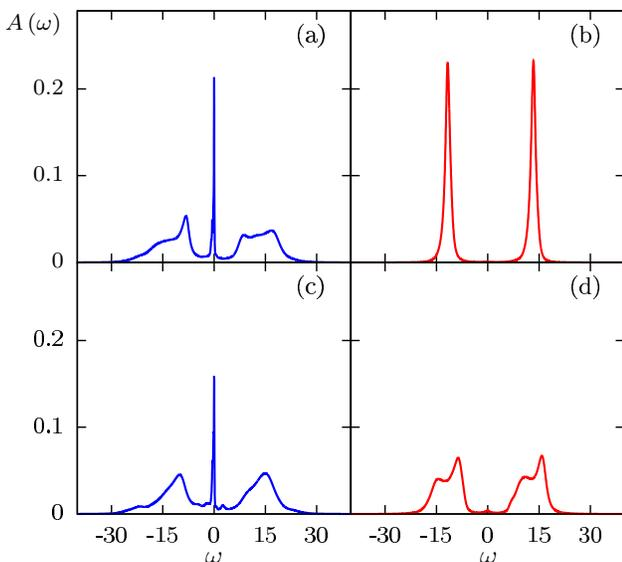
FIG. 4: Local spectral functions  $A_i(\omega, t)$  on four different atoms at a given instant of the DMFT-MD simulations. The Hubbard parameter is  $U = 5.77W_0$ .
