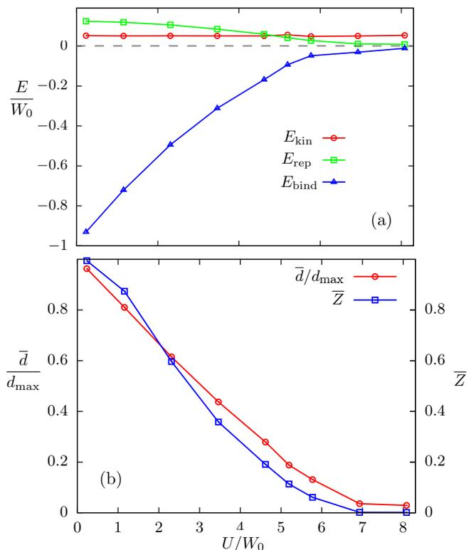
FIG. 1: (a) The various energy densities of the Hubbard liquid model versus the on-site Coulomb repulsion  $U$ . (b) The averaged double occupancy  $\bar{d} = \sum_i d_i/N$  and averaged quasi-particle weight  $\bar{Z} = \sum_i Z_i/N$  as a function of on-site Coulomb interaction  $U$ . The double-occupancy is normalized to its maximum value  $d_{\text{max}} = \langle n_\uparrow \rangle \langle n_\downarrow \rangle = 0.25$  in the uncorrelated state at half-filling.
