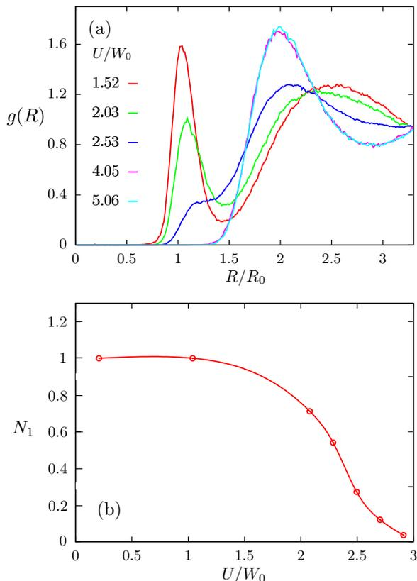
FIG. 9: (a) The pair distribution function  $g(r)$  at different values of Hubbard parameter. The Mott transition occurs at  $U_c \sim 3.1W_0$ . (b) the effective coordination number  $N_1$  versus Hubbard parameter  $U$  obtained from the DMFT-MD simulations.
