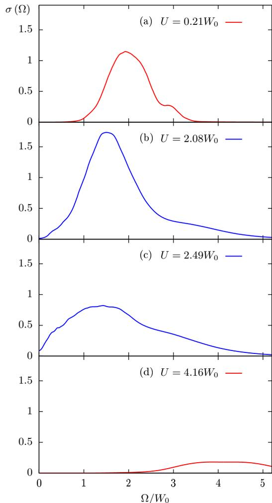
FIG. 10: Time averaged optical conductivity  $\sigma(\Omega)$  as a function of frequency  $\Omega$  obtained from the DMFT-MD simulations. The d.c. conductivity  $\sigma(\Omega \rightarrow 0)$  becomes finite at  $U \sim 2.1W_0$ , signaling the dissociation of dimers and the emergence of the intermediate metallic phase.
