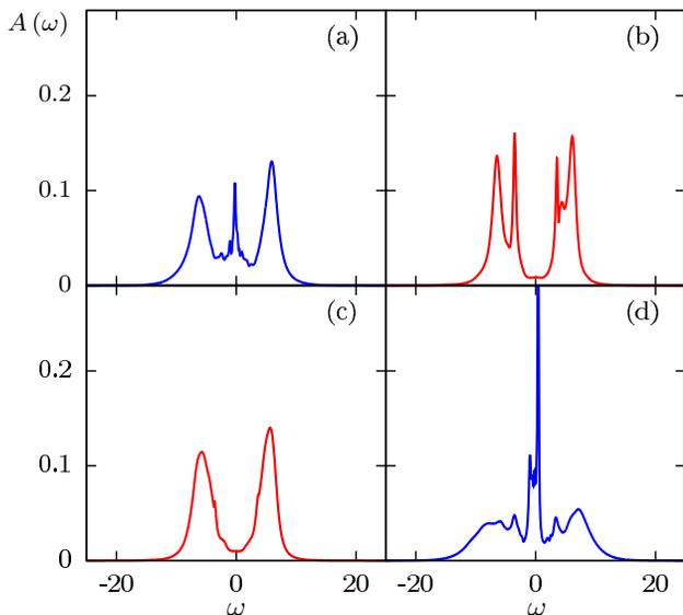
FIG. 11: Local spectral functions  $A_i(\omega, t)$  on four different atoms at a given instant of the DMFT-MD simulations. The Hubbard parameter is  $U = 2.29W_0$ .
