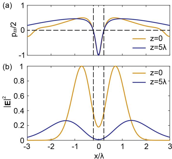
FIG. 3. Cross-sections of the linearly polarised vortex beam with  $w_0 = \lambda$  depicted in Fig. 1 showing (a)  $p_{zz}$  and (b)  $|\mathbf{E}|^2$  at the focal plane and after propagating a distance of  $5\lambda$ . The black dotted guidelines show the points at which  $p_{zz} = 0$ , and the corresponding field intensity for each cross-section plane.
