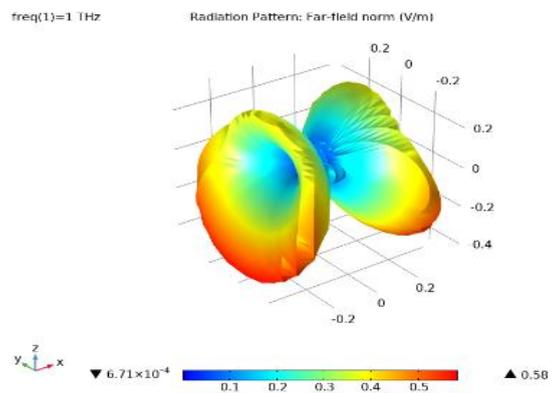
Fig. 2. Numerical simulation of radiation emission pattern at  $f = 1$  THz from a Bi-2212 whisker-based device with a cross-dipole (turnstile) type geometry. The directionality of emission is following the direction of the whisker. This demonstrates antenna-like operation of the whisker (and the electrodes)
