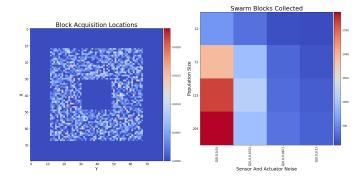
Fig. 6. Demonstration of graphical deliverable generation in stage 4. *Left:* Intra-experiment heatmap showing the average locations where objects are found in the environment (nest in the center). *Right:* Summary performance heatmap showing how the foraging behavior varies under a bivariate batch criteria with changing system size and different levels of sensor and actuator noise.
