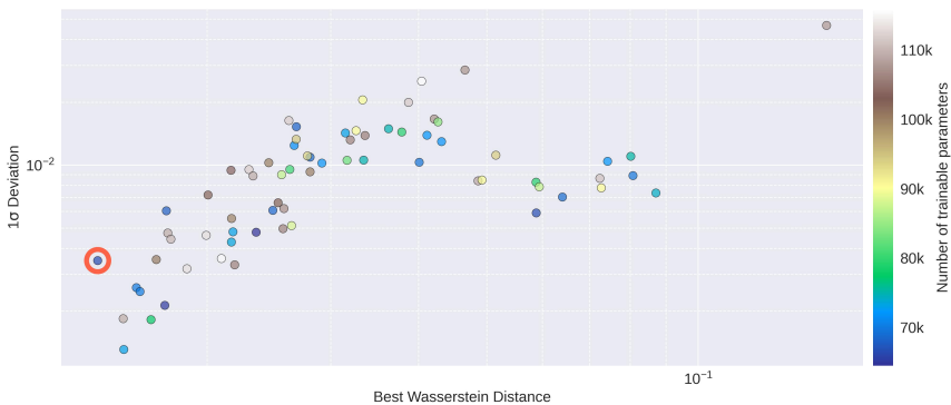
Fig. 6 All 70 solutions obtained with the focus search for case study 1 using the RBF based HPO. Shown are the Wasserstein distance and 1\sigma deviation for all hyperparameters that were sampled as well as the size (complexity) of the corresponding architectures in color. An optimal model was found with a best Wasserstein distance of 0.01398 \pm 0.00349 (circled in red).
