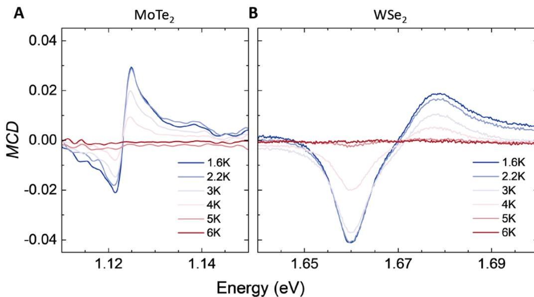
**Supplementary Figure 4 | Temperature dependence of spontaneous MCD spectrum.** **A,B**, MCD spectrum under zero magnetic field for MoTe<sub>2</sub> (**A**) and WSe<sub>2</sub> (**B**) at varying temperatures. The magnitude decreases monotonically with increasing temperature and vanishes between 5 - 6 K.
