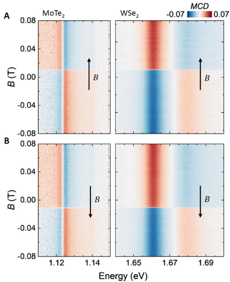
**Supplementary Figure 3 | MCD spectra for magnetic-field range of  $\pm 0.08$  T. A,B,** MCD spectrum as a function of magnetic field between - 0.08 T to 0.08 T in the forward (A) and backward (B) scan directions. The low- and high-energy spectra are dominated by the response of MoTe<sub>2</sub> and WSe<sub>2</sub>, respectively. Hysteric behavior is observed in both layers.
