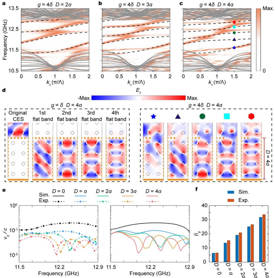
**Fig. 4 | Experimental observation of the broadband topological slow light through higher Brillouin zone winding.** a-c, Experimentally measured (colour) and numerically calculated
