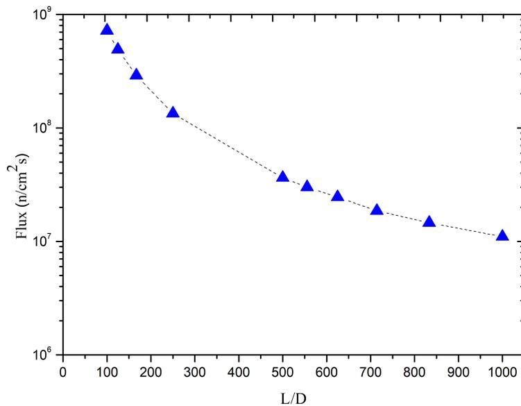
**Figure 9:** Neutron flux in the detector as a function of Neinei resolution. The  $L/D$  range covers all neutron imaging instruments compared.
