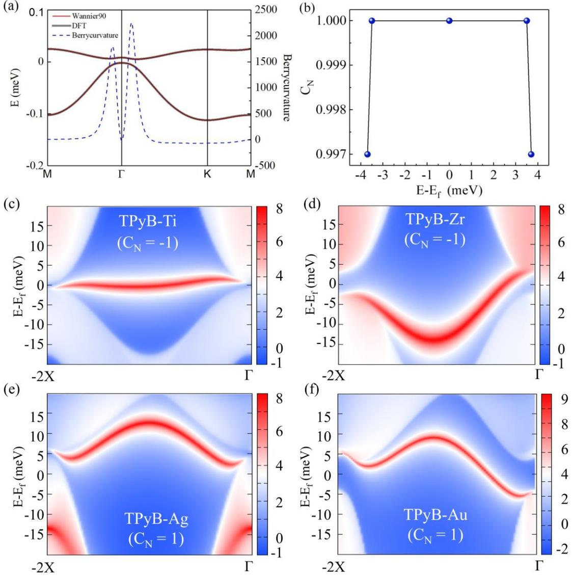
FIG. 3. Topological properties of TPyB-X ( $X=Ti, Zr, Ag, Au$ ). (a) Berry curvature and DFT+SOC calculated band structure along  $M-\Gamma-K-M$  of TPyB-Au. (b) Dependence of Chern number on the position of fermi level in TPyB-Au. (c)-(f) show the chiral edge states of the semi-infinite TPyB-Ti, TPyB-Zr, TPyB-Ag, TPyB-Au, respectively.
