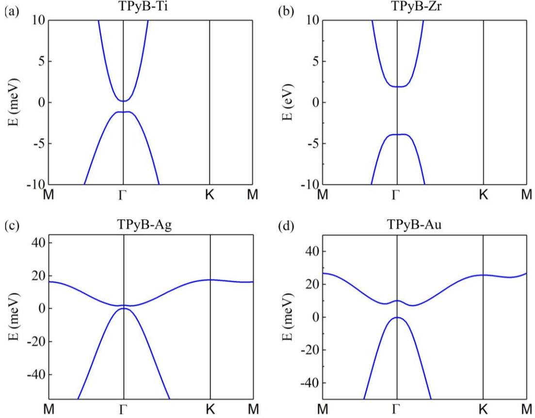
FIG. 2. The DFT+SOC calculated band structures of (a) TPyB-Ti, (b) TPyB-Zr, (c) TPyB-Ag and (d) TPyB-Au, respectively. The Fermi levels are set to zero in (a)-(d).
