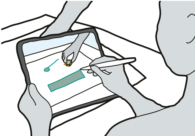
Figure 4: Basic setup of our system. The user draws virtual sketches through the iPad screen and Apple Pencil. After the simple calibration, the embedded 2D canvas onto a table surface in AR can be synchronized with the Sony Toio coordination. The green lines and objects represent the virtually sketched objects whereas a yellow cube object represents the physical Toio robot.
