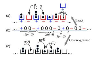
FIG. 1. Mapping lattice model of RTPs to a urn model (misanthrope process) where hop rate of a particle from one urn to the next depends on the total particles present in the departure and the arrival urn. The current J(m) that passes through two consecutive domain having in total m vacant sites, plays the role of hop rate u(m).
