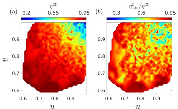
FIG. 2. Results for (a) upper and (b) lower bounds on  $\eta^{(2)}$  for an asymmetrically driven qubit-Otto cycle.  $\omega_0, \omega_1, T_c$  and  $T_h$  were chosen randomly from uniform distribution between the interval  $[0, 5]$ .  $u, v$  were chosen between  $[0, 1]$ . Simulations done over 2.5 million points. The white color regions correspond to situations where the generalized engine conditions *i.e.*,  $\langle W \rangle_F \leq 0$  and  $\langle W \rangle_R \leq 0$  are not satisfied.
