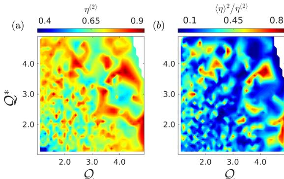
FIG. 5. For an asymmetrically driven HO-Otto cycle (a) upper and (b) lower bounds on  $\eta^{(2)}$  in the engine regime.  $\omega_0, \omega_1, T_c$  and  $T_h$  were chosen randomly from uniform distribution between the interval  $[0,5]$ .  $\mathcal{Q}, \mathcal{Q}^*$  were chosen between  $[1,6]$ . Simulations done over 2.5 million points.
