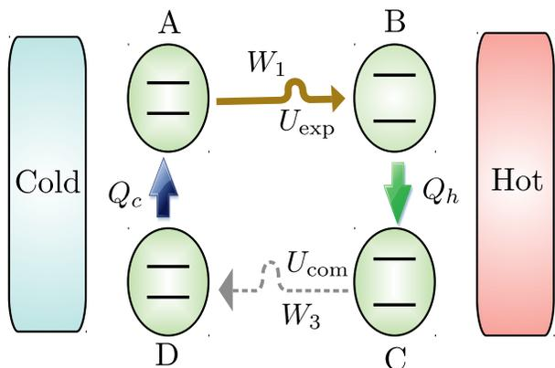
FIG. 1. Schematic for a finite-time asymmetrically driven quantum Otto cycle: Two unitary strokes ( $A \rightarrow B$ ) and ( $C \rightarrow D$ ) correspond to expansion and compression of the working medium and governed by  $U_{\text{exp}}$  and  $U_{\text{com}}$ , respectively. For symmetric driving,  $U_{\text{com}} = \Theta U_{\text{exp}}^\dagger \Theta^\dagger$ . The thermalization strokes are represented by ( $B \rightarrow C$ ) for the hot end and ( $D \rightarrow A$ ) for the cold end.
