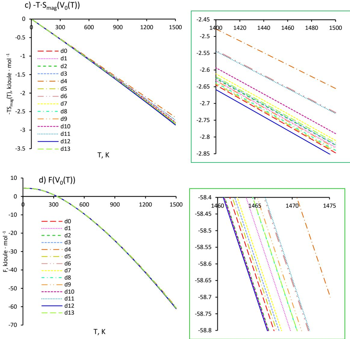
**Figure 8.** The free energy curves  $F(T)$  of  $\text{Co}_7\text{Mo}_6$  and its energy terms calculated for  $d0 \div d13$  routes. a) Electronic energies,  $F_e(V_0(T))$ ; b) Vibrational energies,  $F_{\text{vib}}(V_0(T))$ ; c) Magnetic entropies,  $-T \cdot S_{\text{mag}}(V_0(T))$ ; d) Free energies,  $F(V_0(T))$ . On the right sides of the graphs, in the inserts, magnified values are shown for convenience.
