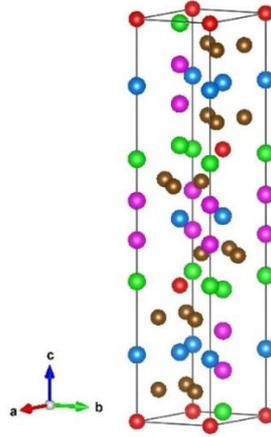
**Figure 1.** Unit cell of  $\text{Co}_7\text{Mo}_6$   $\mu$ -phase, in the hexagonal notation. Co atoms occupy  $3a$  and  $18h$  Wyckoff sites are shown in red and brown respectively while Mo atoms occupy  $6c$ ,  $6c'$  and  $6c''$  sites are shown in blue, green and pink respectively.
