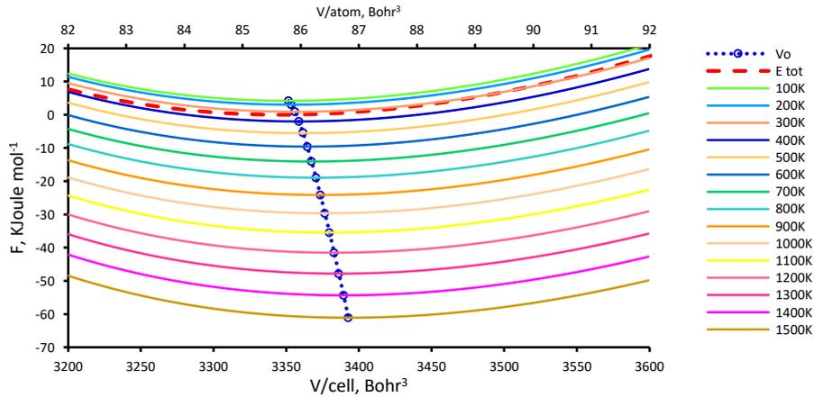
**Figure 7.** Curves of Helmholtz free energy  $F(V, T)$  calculated versus volumes at finite temperatures for  $\text{Co}_7\text{Mo}_6$  along the  $d12$  path. The total energy  $E_{tot}(V)$  is shown by red dashed line. The volume  $V(T)$  is shown by blue dotted line, where open circles denote equilibrium volume.
