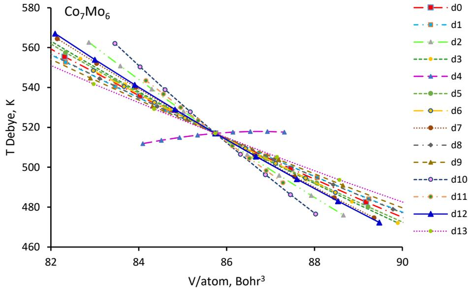
**Figure 5.** Curves of Debye temperatures  $\theta_D(V)$  vs volumes calculated for  $\text{Co}_7\text{Mo}_6$  along the  $d0 \div d13$  routes.
