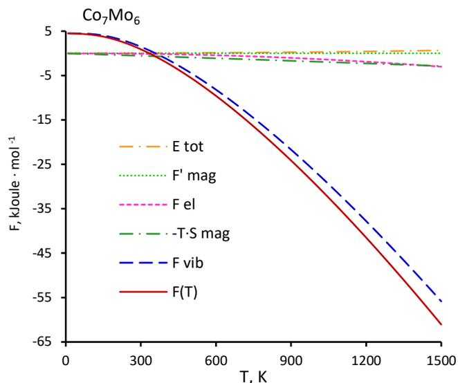
**Figure 9.** The graphs of free energies  $F(V_0(T))$  for  $\text{Co}_7\text{Mo}_6$  with correspondent terms: total, magnetic, electronic, magnetic entropy and vibrational energies calculated along the  $d12$  path.
