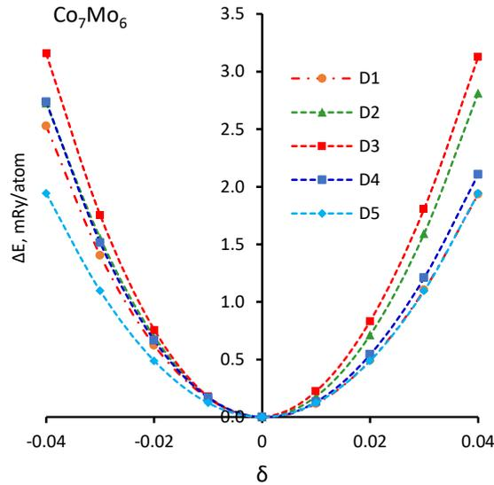
**Figure 2.** The curves of differences in total energies ( $\Delta E = E_{tot}(V, \delta_i) - E_{tot}(V_0, 0)$ , mRy/atom) as functions of applied strains ( $\delta$ ) occurring while imposing the distortion matrices  $D_1 \div D_5$  on the lattice  $\text{Co}_7\text{Mo}_6$ , calculated at  $T = 0\text{K}$ . The dotted lines are approximations of polynomial functions.
