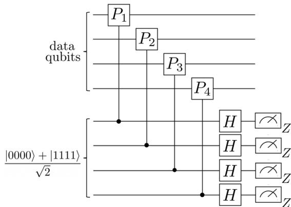
FIGURE 1: Shor syndrome extraction circuit for measuring a stabilizer generator of the form  $M = P_1 \otimes P_2 \otimes P_3 \otimes P_4$ . The ancilla qubits are initially prepared in the cat state  $\frac{1}{\sqrt{2}}(|0000\rangle + |1111\rangle)$  and measured in the  $Z$  basis at the end. Even and odd parities of the measurement results correspond to  $+1$  and  $-1$  eigenvalues of  $M$ .
