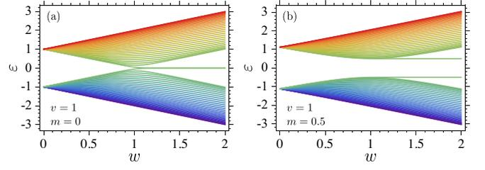
FIG. 1. (Color online) Eigenenergies  $\varepsilon$  calculated as a function of  $w$  for the open RM chain consisting of  $N = 30$  unit cells. Two panels compare the numerical results for (a)  $m = 0$  and (b)  $m = 0.5$ . In these figures,  $v$  is taken as the energy unit ( $v = 1$ ).
