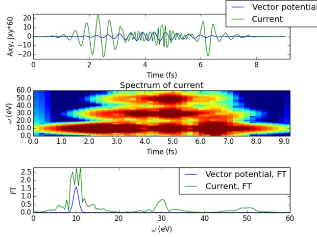
FIG. 8. High harmonic generation on 12-sites chain for Gaussian pulse with central frequency  $\omega = 10$  eV,  $FWHM = 3$  fs, and  $A_0 = 5$ , polarization along the chain. Upper panel: vector potential (blue) and current (green); middle panel: Gabor transform of the current; Lower panel: spectra of incoming pulse (blue) and current (green).
