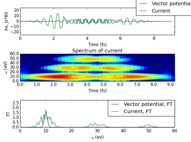
FIG. 7. High harmonic generation on square lattice for gaussian pulse with central frequency  $\omega = 10$  eV,  $FWHM = 3$  fs, and  $A_0 = 5$ , polarization along  $[10]$  direction. Upper panel: vector potential (blue) and current (green); middle panel: Gabor transform of the current; Lower panel: spectra of incoming pulse (blue) and current (green).
