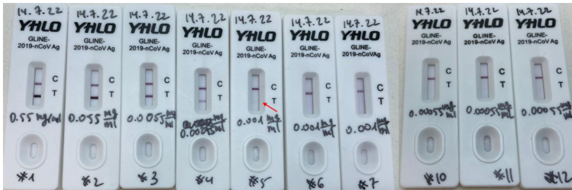
Figure S7 – "YHLO GLINE-2019-nCoV Ag for self-testing" RATs after reaction with different concentrations of nucleocapsid protein. The lowest concentration that showed positive result is 1 \mu\text{g mL}^{-1} ; One out of three RAT showed a weak T-line (red arrow).
