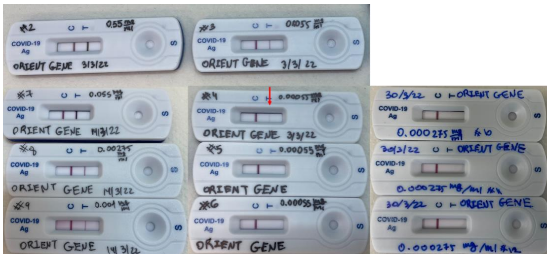
Figure S5 – "Orient Gene Rapid COVID-19 (Antigen) Self-Test" RATs after reaction with different concentrations of nucleocapsid protein. The lowest concentration that showed positive result is 0.55 \mu\text{g mL}^{-1} ; Only one out of three RAT showed a T-line (red arrow).
