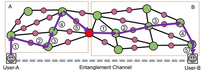
FIG. 5. Hybrid connection model for construction of end-to-end entanglement channel in quantum internet. The red quantum node is the fixed path of connection-oriented protocol. A and B are two connectionless areas connected by red node.
