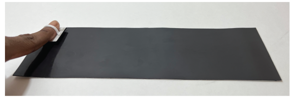
Figure 13: A hand-held token can be programmed to exhibit specific interactions with any location on a programmed sheet.
