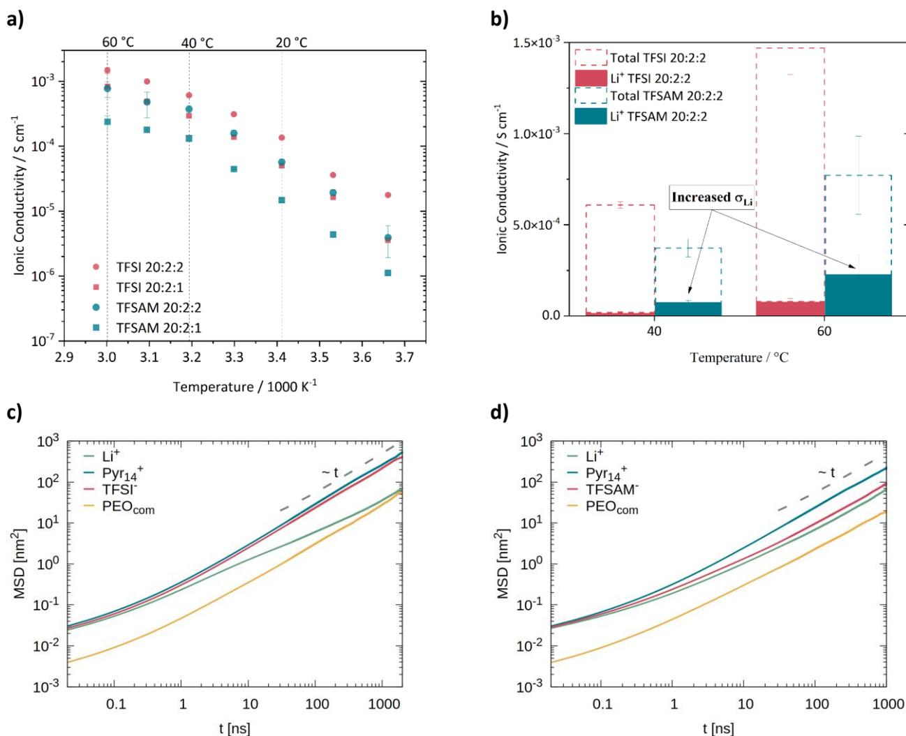
Figure 5: **Top row: a)** Temperature dependent ionic conductivities of TFSAM and TFSI based ternary electrolytes with PEO:salt:IL ratios 20:2:1 and 20:2:2; **b)** total ionic conductivity and portion of the conductivity contributed by  $\text{Li}^+$  at 40 and 60 °C; **bottom row:** mean squared displacements of all molecular constituents in **c)** the TFSI-based and **d)** the TFSAM-based mixture.
