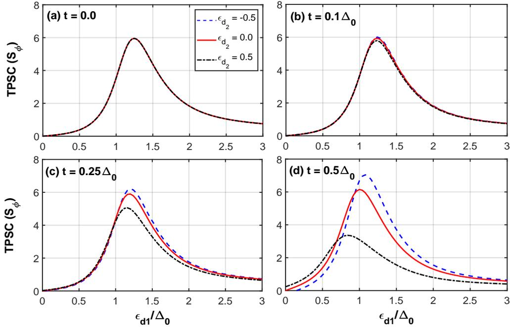
Figure 7: The variation of thermophase Seebeck coefficient ( $S_\phi$ ) with  $QD_1$  energy level  $\epsilon_{d_1}$  for different values of  $QD_2$  energy level  $\epsilon_{d_2}$  and  $t$ . The other parameters are  $U = 0$ ,  $\Gamma = 0.1\Delta_0$ ,  $k_B T = 0.2\Delta_0$ .
