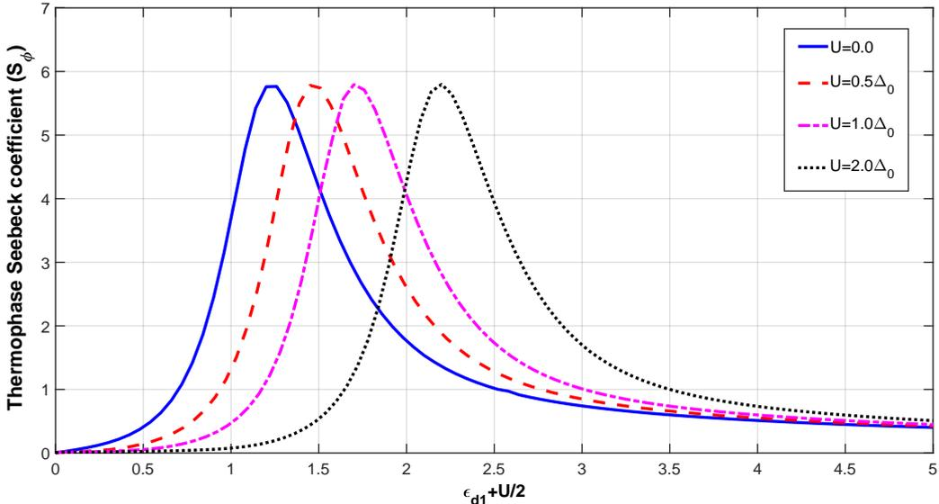
Figure 8: Thermophase Seebeck coefficient as a function of  $QD_1$  energy level for different values of onsite Coulomb interaction. Other parameters are  $t = 0.1\Delta_0$ ,  $k_B T = 0.2\Delta_0$ ,  $\Gamma = 0.1\Delta_0$ ,  $\epsilon_{d_2} = 0.5\Delta_0$
