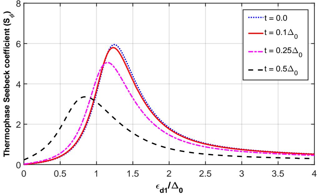
Figure 6: The variation of thermophase Seebeck coefficient ( $S_\phi$ ) with  $QD_1$  energy level  $\epsilon_{d_1}$  for different interdot hopping ( $t$ ). The other parameters are  $U = 0$ ,  $\Gamma = 0.1\Delta_0$ ,  $k_B T = 0.2\Delta_0$ ,  $\epsilon_{d_2} = 0.5\Delta_0$ .
