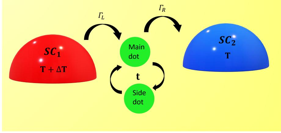
Figure 2: Schematic diagram for double quantum dot in T-shaped geometry coupled with superconducting leads. Main dot ( $QD_1$ ) is directly coupled with superconducting leads while the side dot ( $QD_2$ ) is only coupled with main dot.
