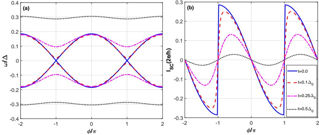
Figure 3: (a) Energy of Andreev bound states and (b) Josephson current as a function of superconducting phase difference ( $\phi$ ) for different value of interdot hopping ( $t$ ) at absolute zero temperature. The other parameters are  $\Gamma = 0.1\Delta_0$ ,  $\epsilon_{d_1} = 0$ ,  $\epsilon_{d_2} = 0.5\Delta_0$ .
