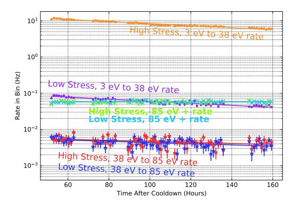
FIG. 3. Time dependence of background rates in High Stress (light colors) and Low Stress (dark colors) calorimeters. Rates are measured in three energy bins: 3–38 eV, 38–85 eV, and 85+ eV. Exponential fits are shown as solid lines. 1 Sigma error bars are shown. Source data are provided as a Source Data file.
