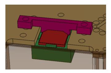
Supplementary Figure S3. **CAD drawing of the LS calorimeter bonding jig design.** Calorimeter (red) is held by 3D printed jigs (bottom, green; top, pink) while being bonded to the copper support plate (gold). An additional element of the housing (bottom half of image) was made semitransparent to more easily show the jig configuration.
