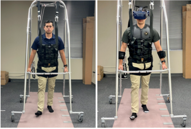
Fig. 4: Participants used harness while performing the timed walking task utilizing the GAITRite system in both the real world (left) and virtual environment (right).
