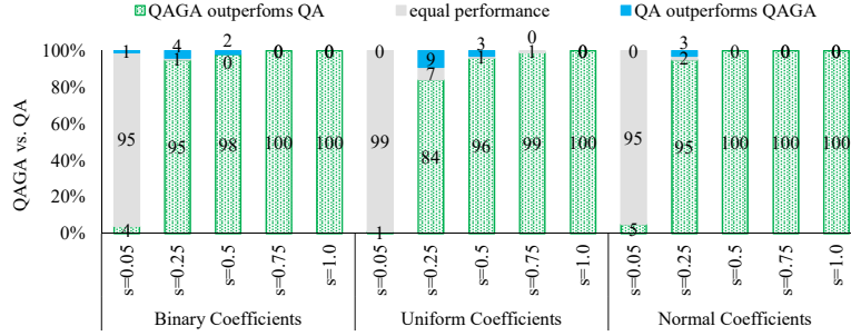
Fig. 1. Performance comparison between QAGA and QA (with spin-reversal-transforms and inter-sample delays) in solving 100 random benchmark problems with N = 50 spin variables and different sparsity rates s
