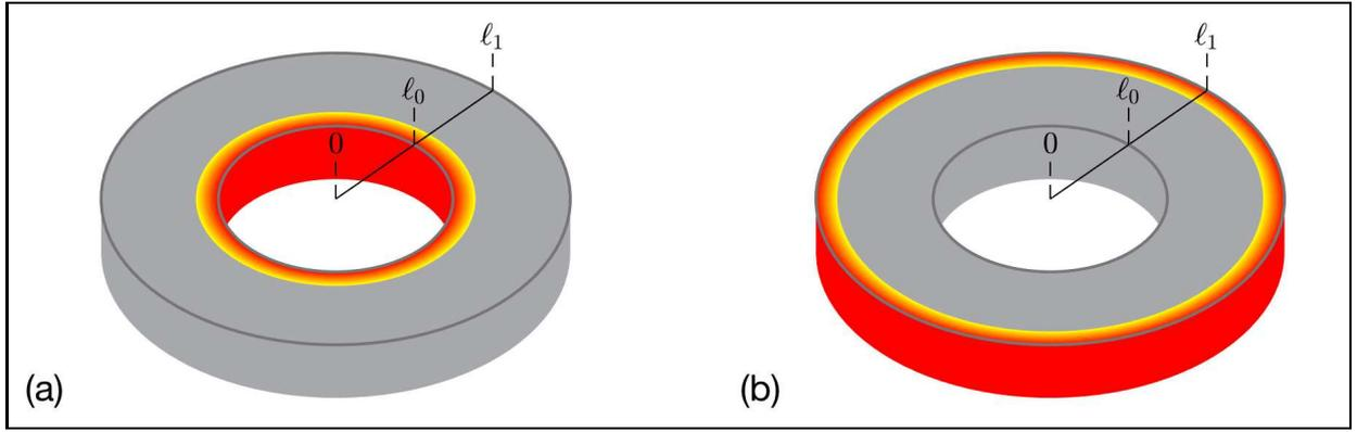
**Figure 1: Cylindrical shell shaped samples.** (a) outward configuration where the heat pulse is applied uniformly on the inner surface ( $x = \ell_0$ ) and the temperature rise is recorded on the outer surface ( $x = \ell_1$ ) and (b) inward configuration where the heat pulse is applied uniformly on the outer surface ( $x = \ell_1$ ) and the temperature rise is recorded on the inner surface ( $x = \ell_0$ ).
