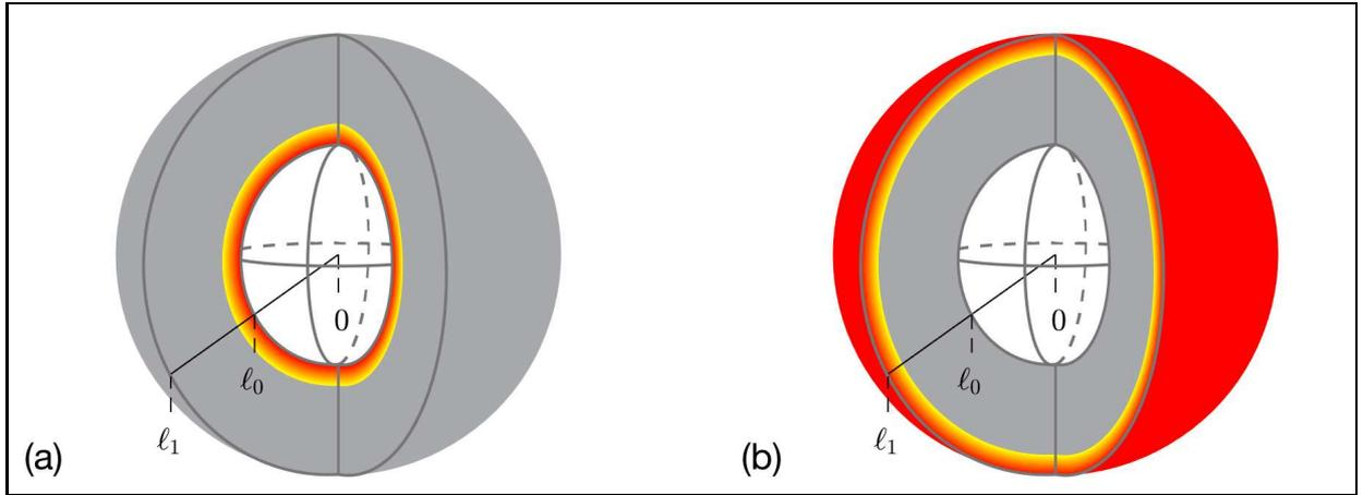
**Figure 2: Spherical shell shaped samples.** (a) outward configuration where the heat pulse is applied uniformly on the inner surface ( $x = \ell_0$ ) and the temperature rise is recorded on the outer surface ( $x = \ell_1$ ) and (b) inward configuration where the heat pulse is applied uniformly on the outer surface ( $x = \ell_1$ ) and the temperature rise is recorded on the inner surface ( $x = \ell_0$ ).
