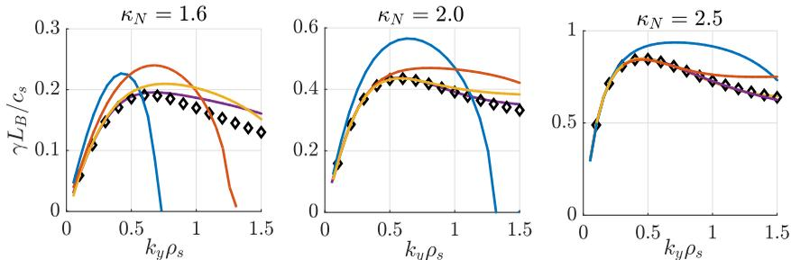
FIGURE 2. Growth rates of the linear entropy mode in the collisionless case ( $\nu = 0$ ) for three different drive values,  $\kappa_N = 1.6$  (left),  $\kappa_N = 2.0$  (middle) and  $\kappa_N = 2.5$  (right), keeping  $\eta = 0.25$ . The growth rates are obtained with GENE with  $N_{v_{\parallel}} = 32$  and  $N_{\mu} = 16$  velocity grid points (black diamonds) and different gyromoment sets: (4, 2) (blue), (10, 5) (red), (20, 10) (yellow) and (30, 15) (purple).
