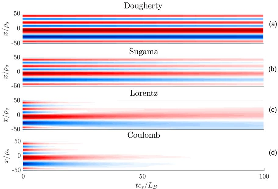
FIGURE 13. Time evolution of the  $y$ -averaged zonal flows profile,  $\langle \partial_x \phi \rangle_y$ , for the Dougherty (a), Sugama (b), Lorentz (c) and Coulomb (d) collision operators, using the saturated state of the collisionless simulation at  $t_0 = 5000$  for  $\kappa_N = 1.6$ ,  $\nu = 0.1$  and  $\eta = 0.25$  as initial conditions.
