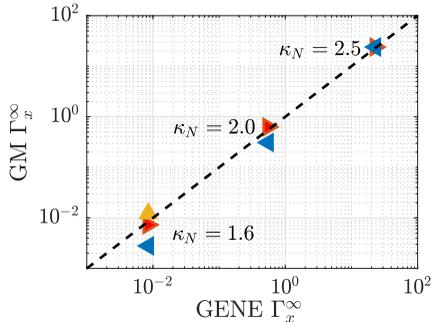
FIGURE 3. Comparison of the time-averaged transport level  $\Gamma_x^\infty = \langle \Gamma_x \rangle_t$  obtained with the gyromoment (GM) approach for  $(P, J) = (4, 2)$  (blue),  $(10, 5)$  (red) and  $(20, 10)$  (yellow) and GENE,  $\eta = 0.25$ . The time traces are presented on Fig. 5.
