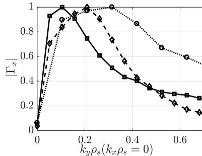
FIGURE 4. Spectrum of the radial particle flux,  $\langle |\Gamma_x(k_x = 0, k_y)| \rangle_t$  for the highest resolution simulations presented in Fig. 6 for  $\kappa_N = 2.5$  (solid squares),  $\kappa_N = 2.0$  (dashed diamonds) and  $\kappa_N = 1.6$  (dotted circles),  $\eta = 0.25$ .
