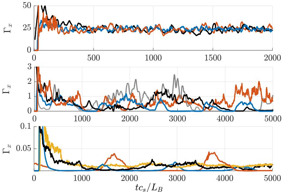
FIGURE 5. Radial particle transport  $\Gamma_x(t)$  (see Eq. (2.21)) from our nonlinear simulations. GENE results are obtained with constant  $\mu_{HD}$  (black) and  $\mu_{HD}$  set by an adaptive hyperdiffusion algorithm (gray). The gyromoment results are shown for  $(P, J) = (4, 2)$  (blue),  $(P, J) = (10, 5)$  (red) and  $(P, J) = (20, 10)$  (yellow). In all cases  $\eta = 0.25$ .
