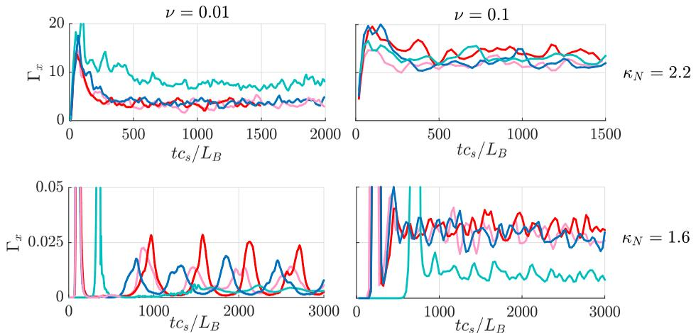
FIGURE 9. Convergence study of the turbulent transport time traces for  $\kappa_N = 2.2$  (top) and  $\kappa_N = 1.6$  (bottom) using the GK Sugama collision operator with  $\nu = 0.01$  (left) and  $\nu = 0.1$  (right). The color indicates the polynomial basis used,  $(P, J) = (2, 1)$  (cyan),  $(P, J) = (4, 2)$  (blue):  $(P, J) = (6, 3)$  (pink),  $(P, J) = (8, 4)$  (red). The other parameters are  $\eta = 0.25$  and  $N_x = 200$ ,  $N_y = 64$  for the spatial resolution.
