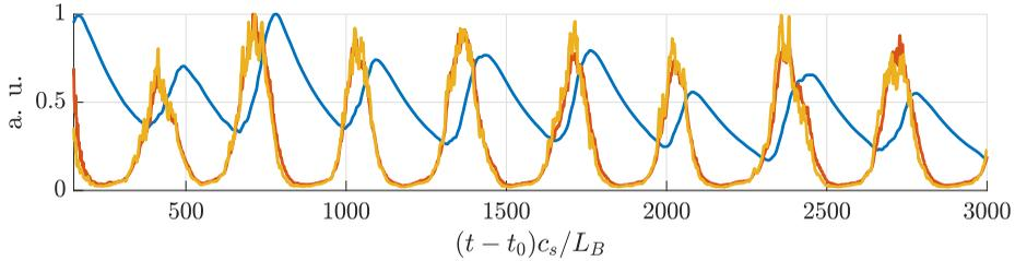
FIGURE 12. Amplitude of the normalized spectral energy for zonal modes ( $\sum_{k_y=0} |\phi_k|$ ; blue), non-zonal modes ( $\sum_{k_y \neq 0} |\phi_k|$ ; red) and transport level ( $\Gamma_x$ ; yellow) obtained for a simulation with the Sugama collision operator for  $\kappa_N = 1.6$ ,  $\eta = 0.25$  and  $\nu = 0.01$ , with  $(P, J) = (4, 2)$  gyromoments
