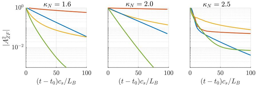
FIGURE 14. Time evolution of  $A_{ZF}^2$  (see eq. 4.1) for the Dougherty (red), Sugama (blue), Lorentz (yellow), and Coulomb (green) collision operators used in the gyromoments approach with a  $(4, 2)$  Hermite-Laguerre basis. The ZF initial conditions are the ones obtained from the  $\kappa_N = 1.6$  (left),  $\kappa_N = 2.0$  (middle), and  $\kappa_N = 2.5$  (right) collisionless simulations. In all cases  $\eta = 0.25$ .
