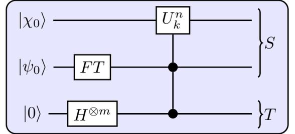
FIG. 1. Schematic circuit representing the generation of the history state (18) through Eq. (13): The Quantum Fourier Transform (FT) is applied to the initial position state  $|\psi_0\rangle$ , while  $H^{\otimes m}$  denotes the Hadamard operator over  $m$  qubits with  $2^m = N$ , such that  $H^{\otimes m} |0\rangle = \frac{1}{\sqrt{N}} \sum_{n=0}^{N-1} |n\rangle$ . Finally the controlled- $U$  gate  $U_k^n$  acts over the initial spin state  $|\chi_0\rangle$ .
