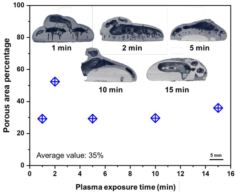
**Figure S.3.** Porous area percentage of the samples partially reduced under hydrogen plasma.
