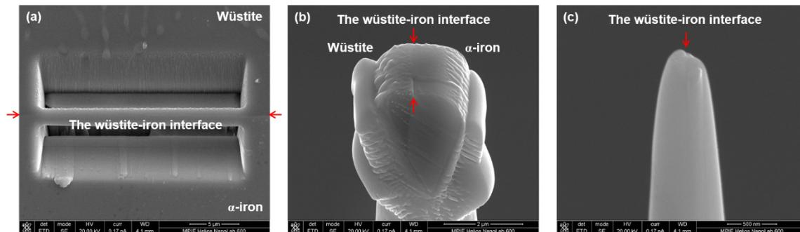
**Figure S.2.** Precision site-specific sample preparation for atom probe tomography tips: (a) wedge milled along the wüstite-iron interface of the 5 min-reduced sample; (b) lift-out sample on the pre-fabricated Si micro-post for annular milling; (c) APT tip before the final annular milling step.
