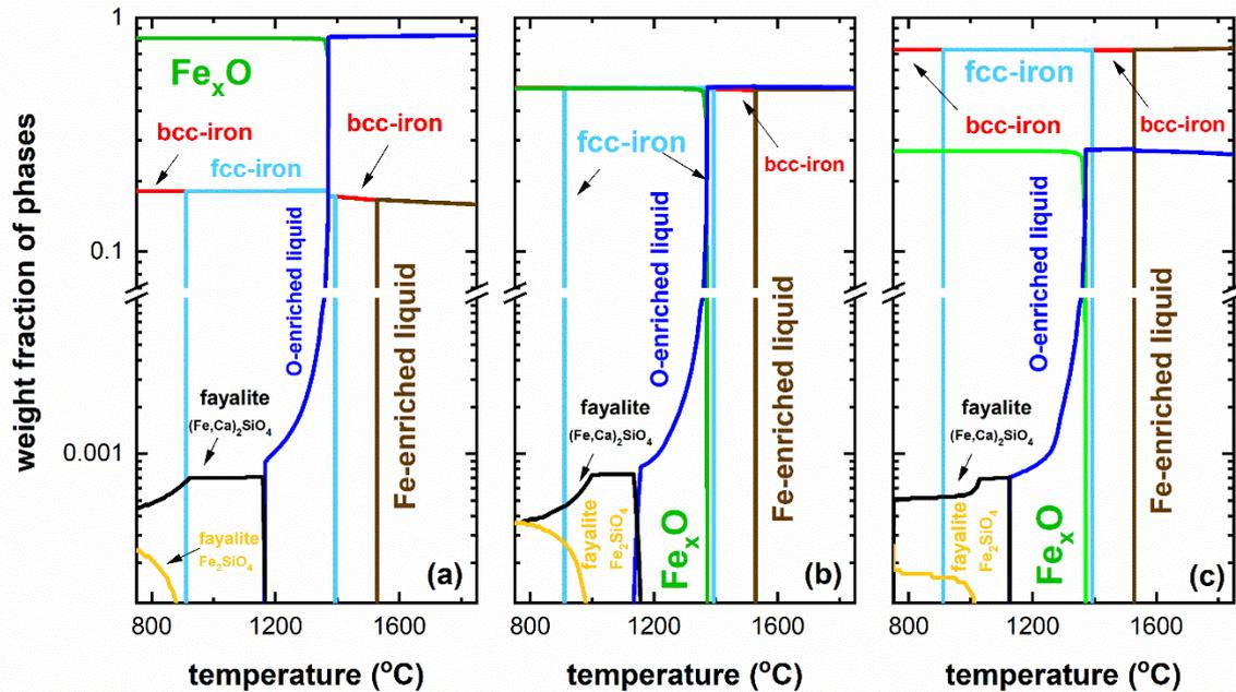
**Figure S.1.** Phase equilibrium calculations for the samples partially reduced for (a) 5 min, (b) 10 min and (c) 15 min, conducted using the software ThermoCalc with the aid of the metal oxide solutions database TCOX10.
