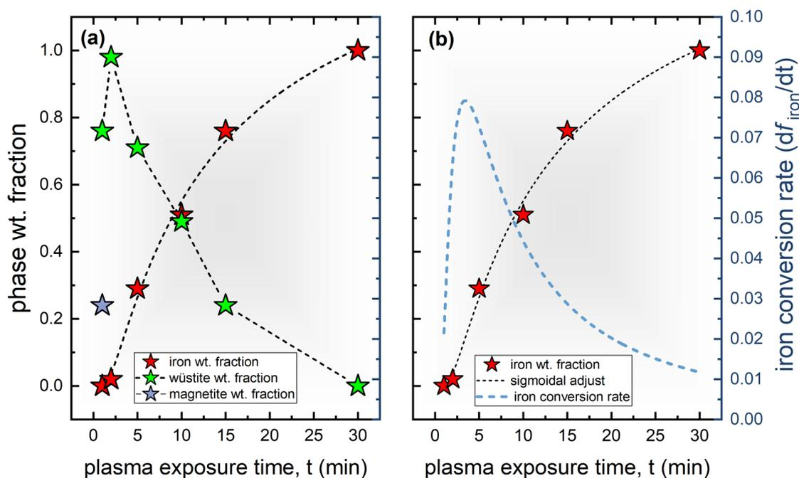
**Figure 10.** Phase transformation kinetics during hydrogen plasma-based reduction of the 9 g-hematite pieces. (a) Changes in the phase weight fractions of magnetite, wüstite, and ferrite. (b) Iron conversion kinetics and corresponding transformation rates.
