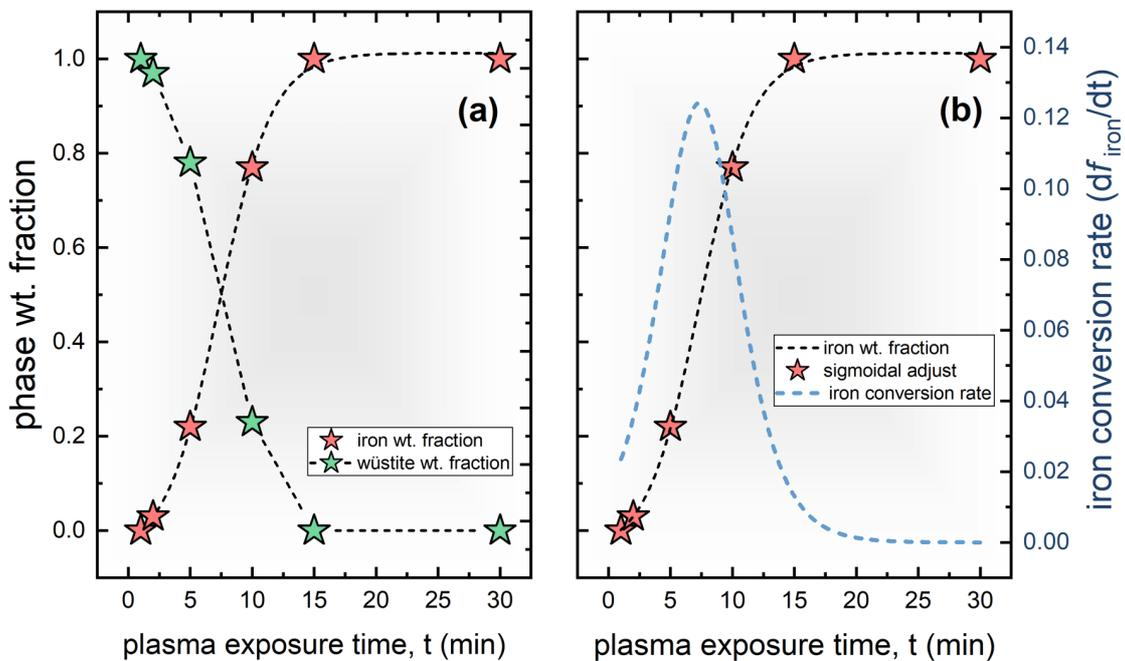
**Figure 12.** Phase transformation kinetics during hydrogen plasma-based reduction of the 15 g-hematite pieces. **(a)** Changes in the phase weight fractions of magnetite, wüstite, and ferrite **(b)** Iron conversion kinetics and corresponding transformation rates.
