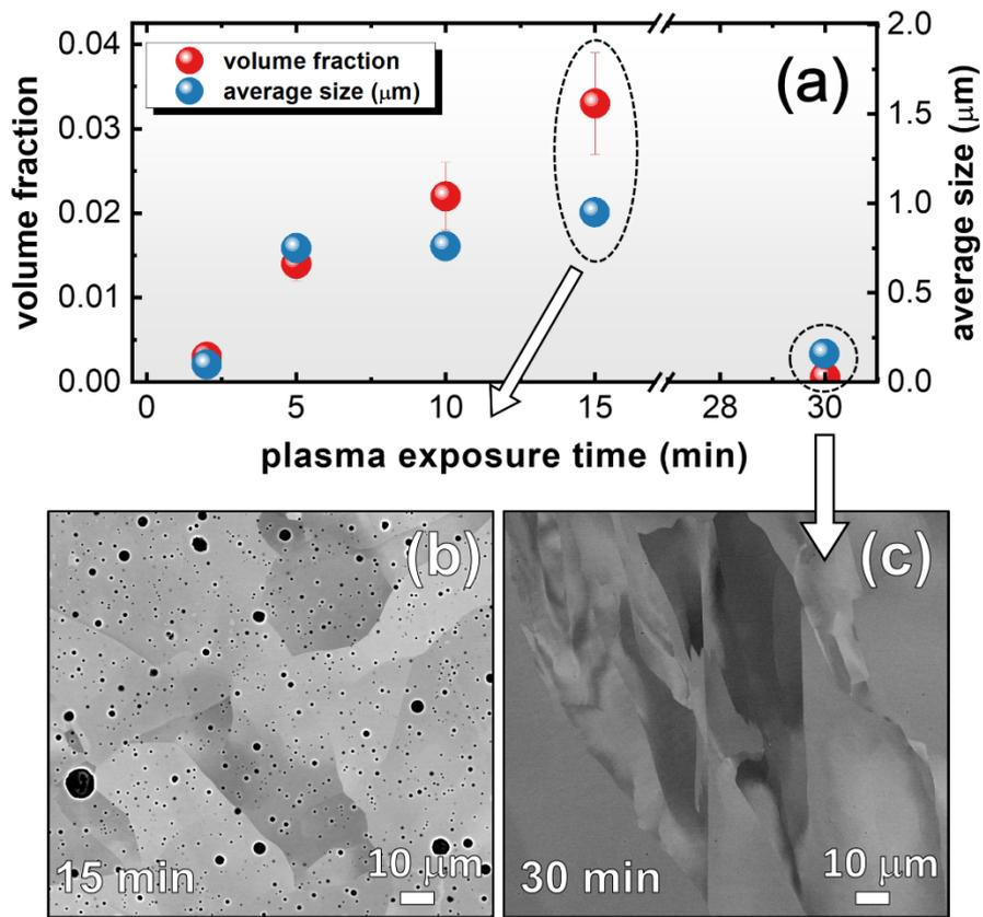
**Figure 7.** (a) Evolution of the volume fraction and average size of the oxide particles pinned inside iron. (b) ECCI-image of the microstructure of the iron formed in the 15-min partially reduced sample (c) ECCI-image of the sample completely reduced after 30 min of exposure to the hydrogen plasma.
