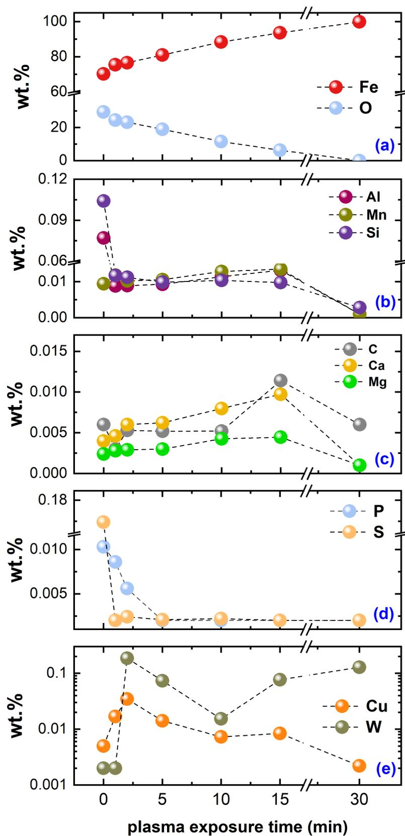
**Figure 8.** Chemical composition evolution during reduction. Changes in weight percentage in terms of (a) Fe and O; (b) Al, Mn, and Si; (c) C, Ca, and Mg; (d) P and S; (e) Cu and W, where the logarithmic y-axis serves to facilitate the visualization.
