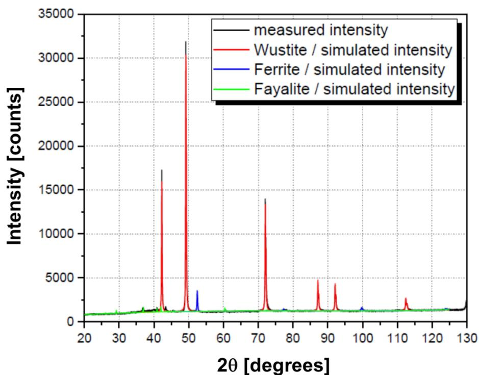
**Figure S.6.** Representative diffractogram of the sample partially reduced for 10 min. The black line represents the experimentally determined data. The red, blue, and green lines represent wüstite, ferrite and fayalite deconvoluted peaks, obtained after Rietveld refinement.
