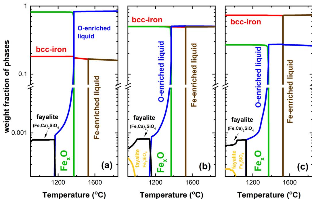
**Figure 9.** Metastability calculations for the samples partially reduced for (a) 5 min, (b) 10 min and (c) 15 min, conducted using the software ThermoCalc with the aid of the metal oxide solutions database TCOX10. For the construction of these diagrams, austenite (fcc-iron) was excluded from the calculations.
