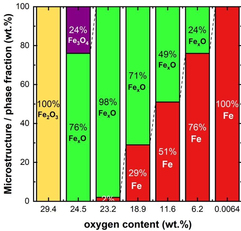
**Figure 11.** Diagram ‘microstructure versus oxygen content’ for the 9 g-hematite pieces reduced via hydrogen plasma under different exposure times.
