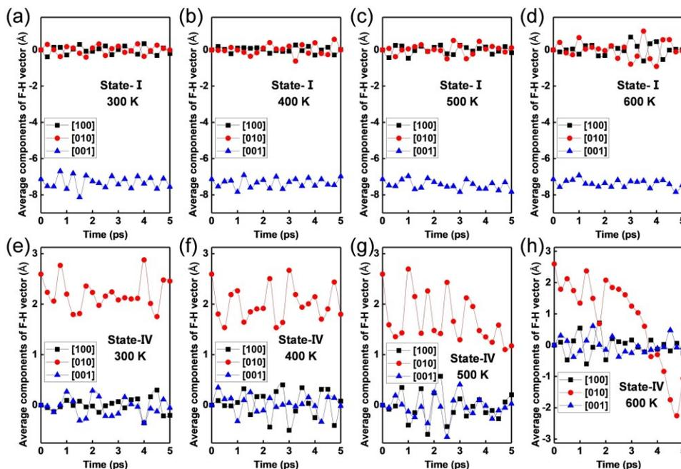
Figure 5. Thermal stability of ferroelectricity of state-I and state-IV of  $\text{Cr}(\text{h-fpyz})_2$  monolayer. (a)-(d) Fluctuation of the average components of the F-H vector as a function of simulation time for
