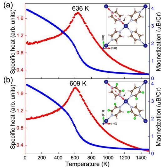
Figure 2. Specific heat (in red) and magnetic moment per Cr ions (in blue) of (a) Cr(py<sub>2</sub>)<sub>2</sub> and (b) state-I of Cr(h-fpyz)<sub>2</sub> monolayer as a function of temperature, from Monte Carlo (MC) simulation. The inset shows the interactions between the Cr ions considered in the present spin Hamiltonian model.
