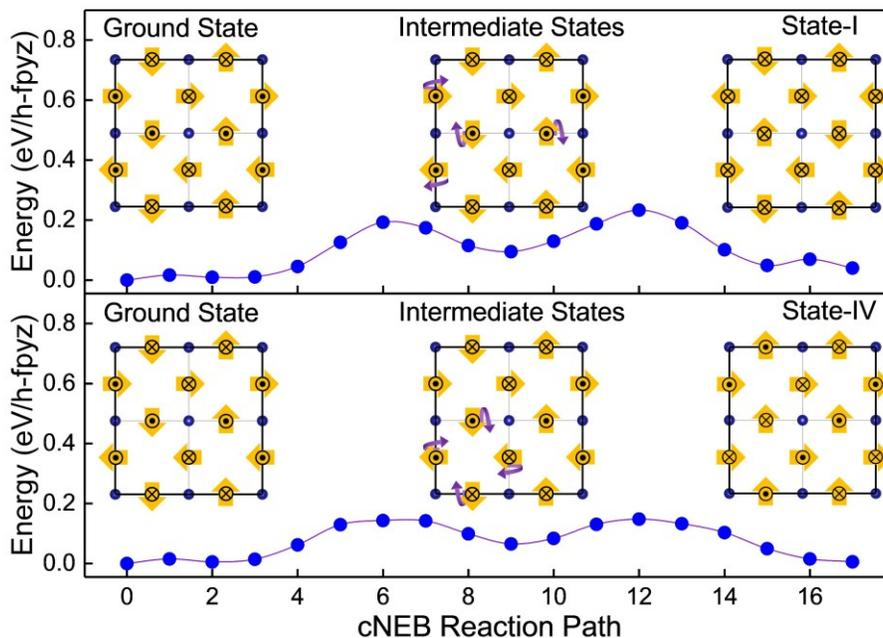
Figure 6. Transition paths between the ground state of  $\text{Cr}(\text{h-fpyz})_2$  monolayer and its state-I and IV, respectively. The h-fpyz molecules with positive and negative out-of-plane dipole components are indicated by orange arrows with dots and crosses, respectively, for clarity. The purple cycle arrows in the insets represent the rotation of h-fpyz molecules during the phase transitions.
