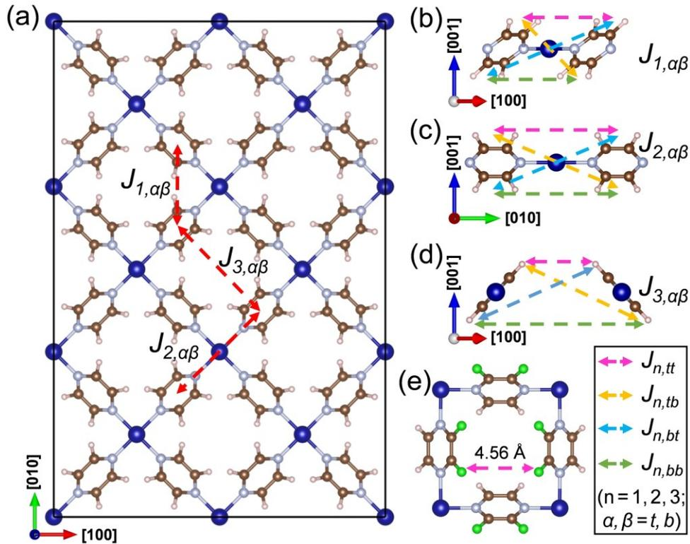
Figure 4. Schematic of the interactions between molecules considered in the MC simulation. (a) The nearest-, next nearest- and third nearest-neighboring interactions between molecules. (b)-(d) Detailed illustration of the interaction parameters  $J_{n,\alpha\beta}$  between two molecules. (e) Closest distance arrangement between F atoms on the third nearest-neighboring h-fpyz molecules of optimized state-I.
