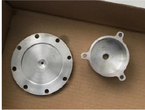
Figure 3: The plasma (left) and ground (right) electrodes
