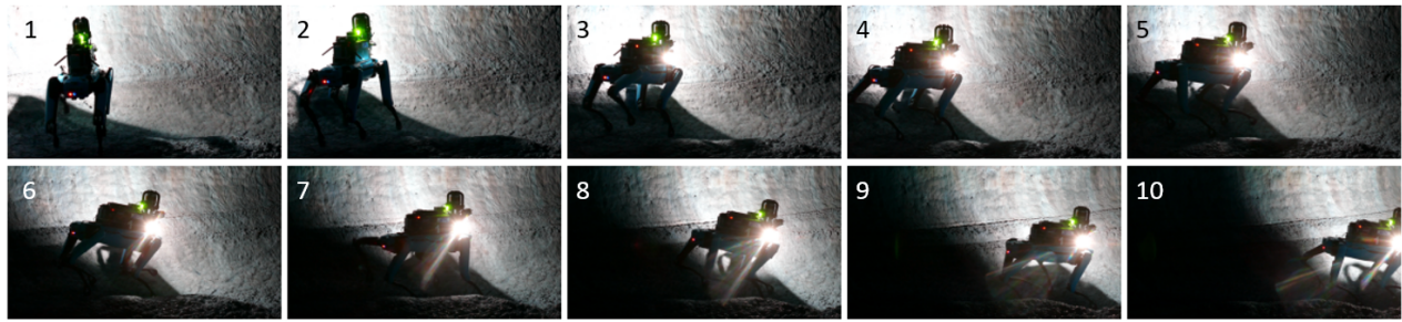
Fig. 8. Time series of frames showing the Spot robot in crawl mode during field deployment near a sloped surface in a cave after detecting a slip event.
