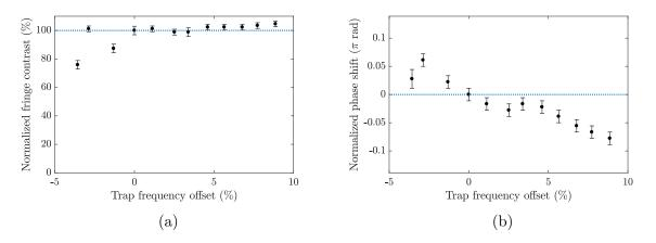
Figure 11: Effect of the trap frequency on the resulting Ramsey fringe contrast (a) and phase shift (b) of the AXY gate. The axial trap frequency is varied, deliberately inducing a mismatch between the pulse timings of the AXY sequence and the motional frequencies. An AXY-16 sequence is applied to generate a  $\frac{\pi}{4}$  phase gate, the dashed line indicates the reference setting of  $\nu_t = 2\pi \times 115$  kHz, to which all results are normalized.
