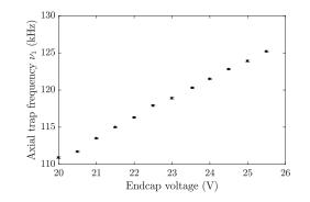
Figure 10: Measurement of the trap frequency. Changing the voltage applied to the endcap electrodes, the axial trapping potential and hence axial motional frequencies are varied. A tickling method using a small AC voltage to excite the ion motion is used to determine the respective trap frequencies.
