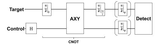
Figure 5: RF sequence for a Bell state measurement. A Hadamard gate is applied to the control qubit to create an equal superposition state, then the AXY sequence framed by two  $\frac{\pi}{2}$  pulses with phases 0 and  $\frac{3\pi}{2}$  creates a CNOT gate. Additional rotations to each qubit are optionally applied for rotating the measurement basis before state read-out.
