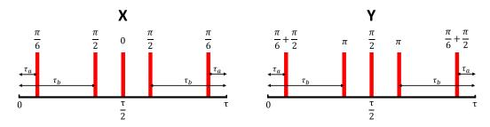
Figure 2: Building blocks of the adaptive XY decoupling sequence. Each block consists of a series of five non-equidistant  $\pi$  pulses, distributed by the block duration  $\tau$  and the pulse positions  $\tau_a$  and  $\tau_b$ . Numbers above the pulses indicate the respective phases within each block, which provide robustness to pulse errors.
