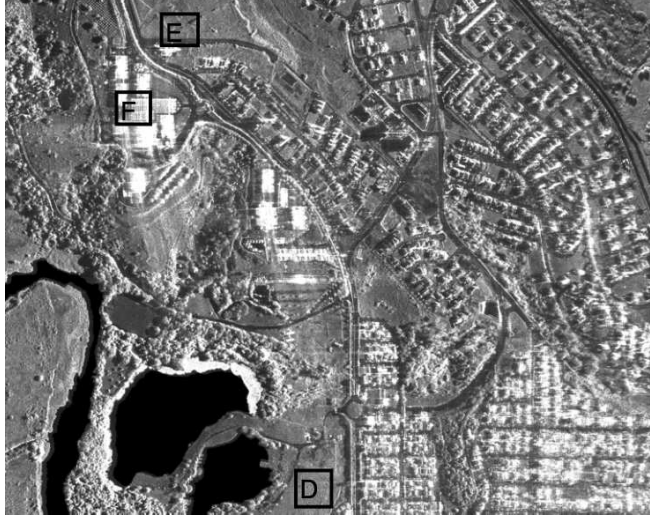
Figure 4: OrbiSAR image used in the regression models showing the tested regions. Regions D, E, and F represent an open area, a road, and an urban land type, respectively.
