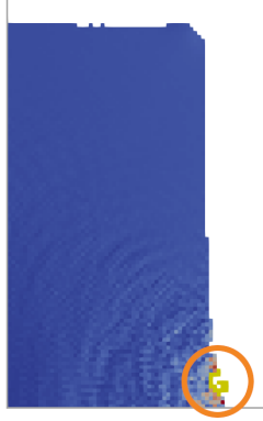
Figure 8: Contour of the simulated rectangular dam break with an initial dam width of W = 50 lattice cells and EXT refilling scheme. At non-dimensionalized time t^* \approx 0.43 , the simulation became numerically unstable. These instabilities were caused by the lattice velocity exceeding the lattice speed of sound c_s in the area marked with the orange circle.
