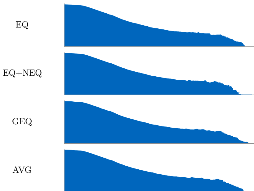
Figure 7: Contour of the simulated rectangular dam break at time t^* = 3 with an initial dam width of W = 200 lattice cells with the EQ (a), EQ+NEQ (b), GEQ (c), and AVG (d) refilling schemes. The simulation with the EXT refilling scheme is not included here because the simulation was numerically unstable. There are noticeable differences between the individual refilling schemes. Owing to the lack of reference data, no accuracy assessment could be made for the contours.
