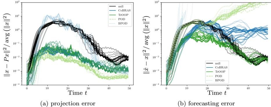
FIG. 4. In (a) we show the reconstruction error using the different linear projections along each testing trajectory. The “null” projection means  $Px = 0$ . In (b) we show the error of the predictions made by the Petrov-Galerkin ROMs. The “null” forecast means  $\hat{x} = 0$ . In (a) and (b) we normalize the errors by the mean kinetic energy along each trajectory. The opacity of the trajectories increases with  $\text{avg}(\|x\|^2)$ .
