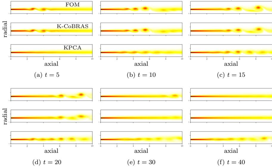
FIG. 8. Snapshots of predicted vorticity in the jet flow using learned 15-dimensional models in kernel feature space along the most energetic testing trajectory, which had impulse magnitude  $u_0 = 0.0938$ .
