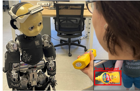
Fig. 1. Target human robot interaction setup. The iCub is tracking the shown object by following the teacher’s hand, while acquiring training samples automatically annotated with the proposed approach.
