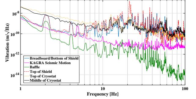
FIG. 11. Vibration spectra of various components considered during Newtonian noise estimation.
