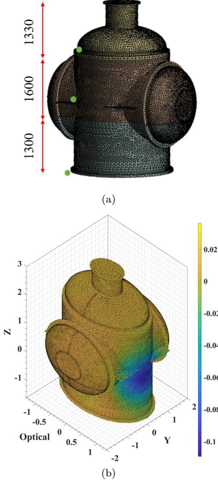
FIG. 8. (a) Mesh generated for cryostat with 124,795 elements. Cryostat was split into three parts and the green dots represent the position where vibrations  $u_{top}$ ,  $u_{middle}$  and  $u_{bottom}$  were measured. (b) 3-D scatter plot where each dot represents an element  $n$  from cryostat mesh while the color is value  $S_{n_{cryostat}}$  of that element in eq. (24)
