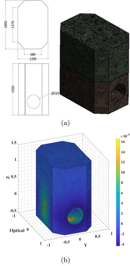
FIG. 7. (a) Mesh generated for outer shield with 262,889 elements each weighing 1.97 g. 2-D drawing showing top and front view of 80K shields. (b) 3-D scatter plot where each dot represents an element  $n$  from outer shield mesh while the color is value  $S_{n_{80K}}$  of that element in eq. (22).
