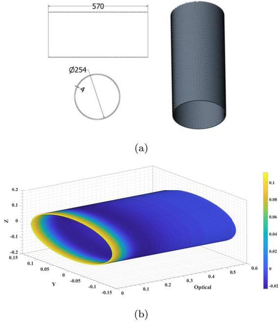
FIG. 5. (a) Mesh generated for baffle. The cylinder is divided into 29,601 elements each weighing 0.24 grams. (b) 3-D scatter plot where each dot represents an element  $n$  from baffle mesh while the color is value  $S_{n_{baffle}}$  of that element in eq. (16)
