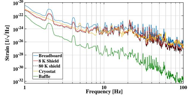
FIG. 9. Comparison of Newtonian Noise strain spectral density from each component, the largest contribution comes from breadboard followed by radiation shields, cryostat and baffle. Note that the force on Test Mass due breadboard/radiation shields and cryostat/baffle are in opposite directions.
