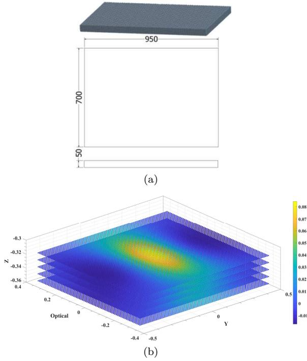
FIG. 3. (a) Mesh generated and 2-D drawing for the breadboard. The cuboid is divided into 33,250 elements each weighing 2.634 grams. (b) 3-D scatter plot where each dot represents an element  $n$  from breadboard mesh while the color is value  $S_{n_{breadboard}}$  of that element in eq. (11)
