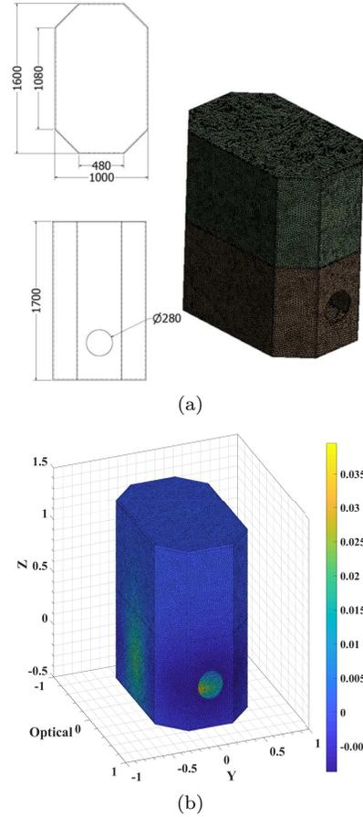
FIG. 6. (a) Mesh generated for inner shield with 200,935 elements each weighing 2.4 g. 2-D drawing showing top and front view of 8K shield. (b) 3-D scatter plot where each dot represents an element  $n$  from inner shield mesh while the color is value  $S_{n_{8K}}$  of element in eq. (19)
