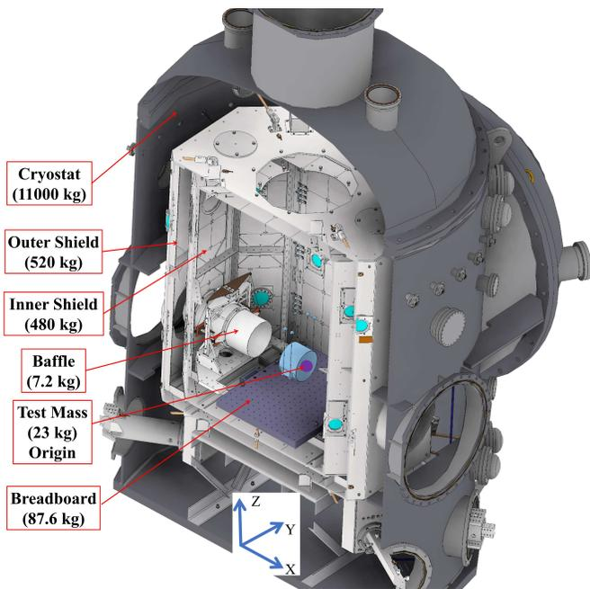
FIG. 2. Coordinate system and summary of components considered in Newtonian noise calculation. Cross-section of KAGRA cryostat showing the components (chamber, baffle, breadboard, inner shield and outer shield) considered for Newtonian noise calculation. The blue arrows denote the coordinate system. The test mass is considered as a point mass, located at origin as denoted by the purple dot.
