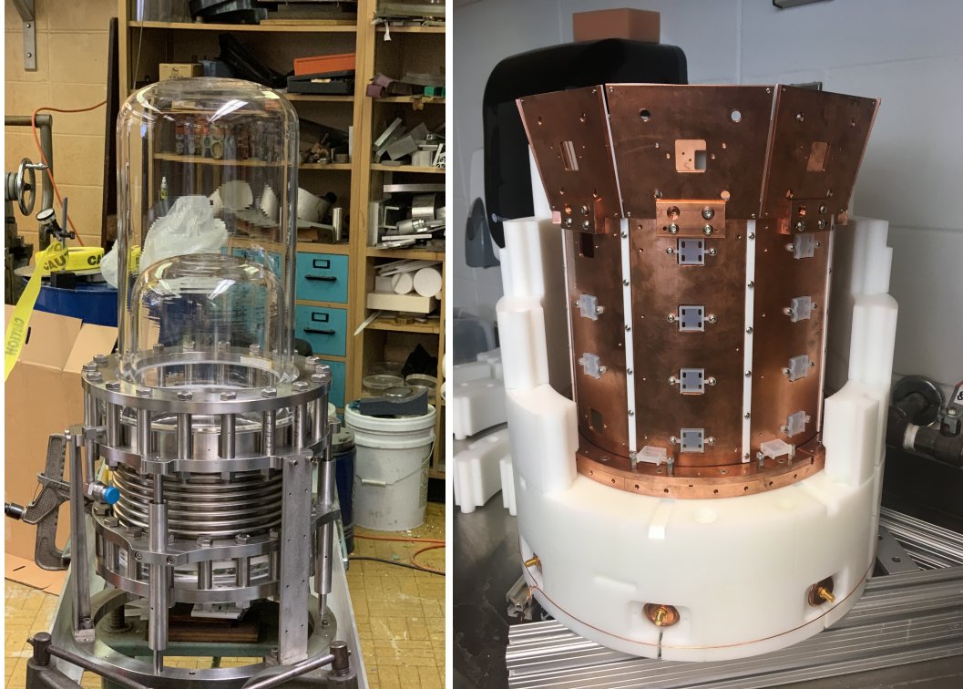
Figure 7: Left: Test of the SBC-LAr10 “inner assembly” comprising the inner and outer fused silica vessels, stainless steel bellows, bellows guides and support structure, and spring-energized PTFE silica-to-metal seals. Right: The partially-assembled HDPE “castle” isolating the warm (superheated) target region from the cold (stable) region, enclosing the copper SiPM support structure that surrounds the target volume. At the bottom of the castle, three of the eight piezoelectric acoustic sensors are visible.
