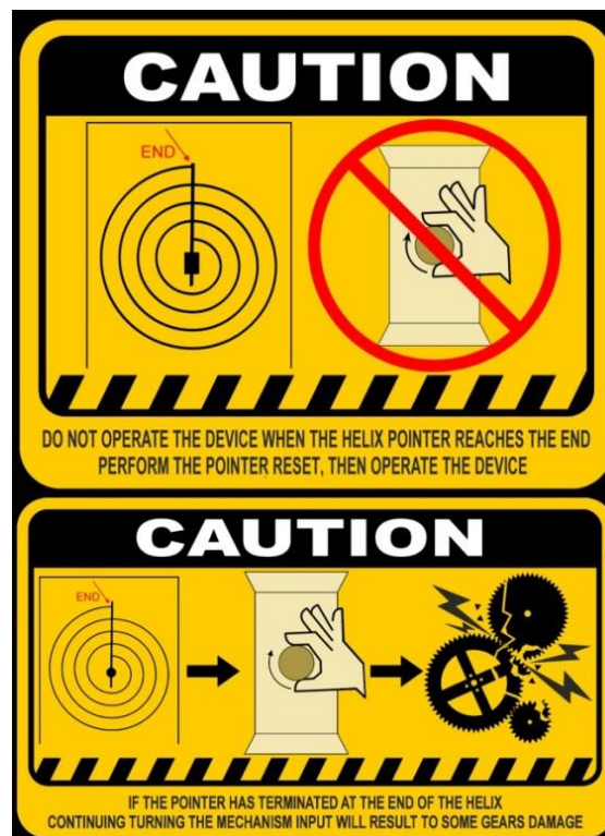
Figure 9: Two of the Caution signs on the Antikythera Mechanism Instruction Manual, in modern terms. The signs of ⚠CAUTION warn the User of the Antikythera Mechanism to take appropriate action: Do not operate the Mechanism if the helix pointer reaches the end, in order avoid the destruction of a number of gears (destruction of their teeth). Idea, design and scheme by the authors.
