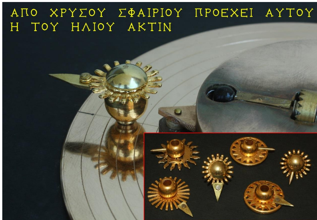
Fig. 10. From the Golden Sphere the Solar Ray (pointer of the Sun) it protrudes. This travels through the three orbits of the superior planets Mars, Jupiter and Saturn. The Lunar pointer travels through the circumferences of Mercury and Venus (see §6.a.). Insert, different designs of the part ΧΡΥΣΟΥΝ ΣΦΑΙΡΙΟΝ with ΗΛΙΟΥ ΑΚΤΙΝ, were constructed by the first Author. Material and image by the Authors
