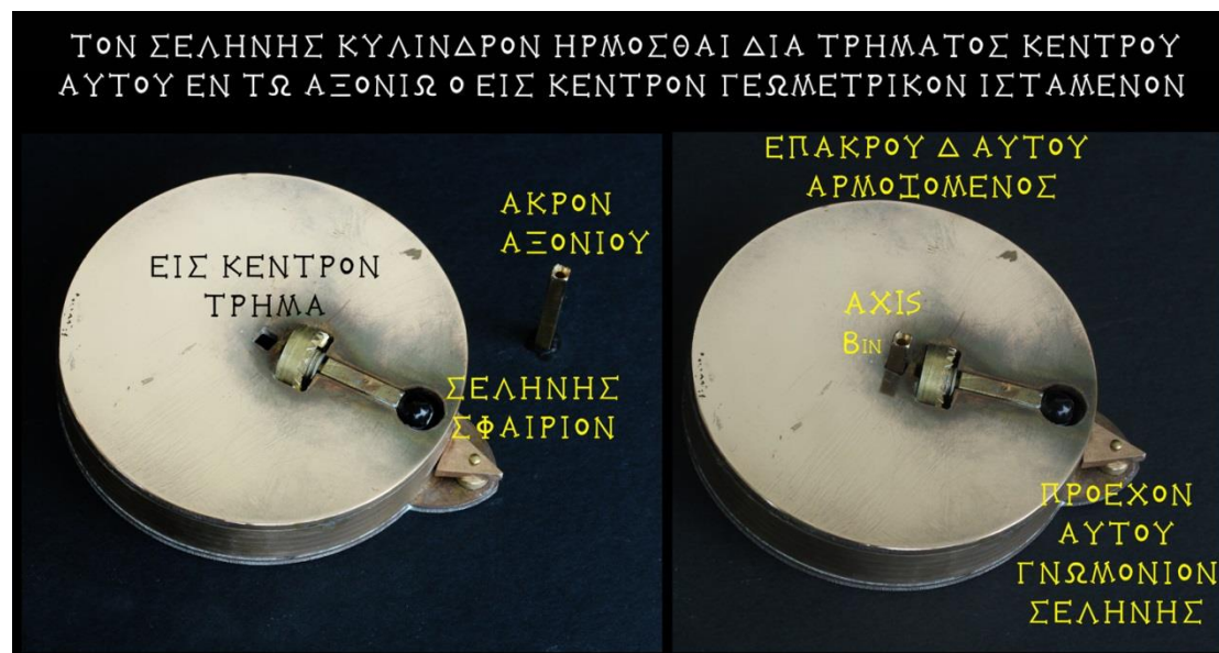
Fig. 5. The Lunar Disc/Cylinder adaptation on the \alpha axis- b_{in} , which is located on the geometrical center of the Mechanism front face. The parts of the Lunar Disc/Cylinder are visible: the Lunar phases sphere and the Lunar pointer. At the center of the disc, the square central hole (ΤΡΗΜΑ) is also visible.
