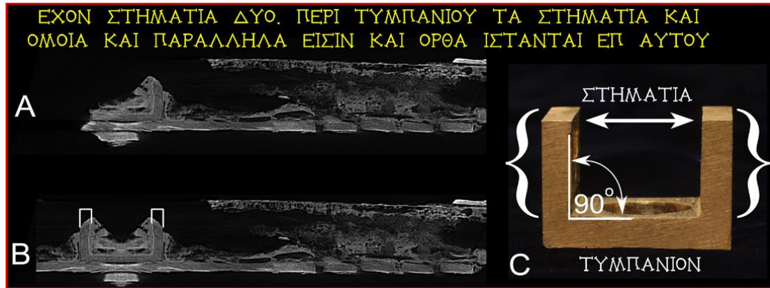
Figure 4: A) AMRP tomography of a part of Fragment B (sagittal view), presenting the profile of the Metonic pointer bearings (ΣΤΗΜΑΤΙΑ), which are parts of the Base (ΤΥΜΠΑΝΙΟΝ). The Volume Data was aligned to the Base direction. B) For the digital reconstruction of the lost parts, the central/axial Symmetry was applied and the profile of the bearings is revealed (see also Anastasiou et al., 2014). The white lines show the probable height of the bearings, as today these parts are missing. The AMRP Computed Tomography was processed by the authors and was taken from the Raw Data Volume, using the software VolviCon. C) The reconstructed Base of the pointer with its bearings in bronze (spare part), by first author.
