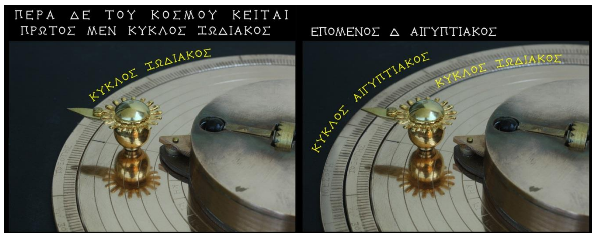
Fig. 13. Beyond Cosmos, there is the Zodiac month ring which is the Ecliptic Sky of the Mechanism. The Egyptian calendar ring follows. Material and image by the Authors
