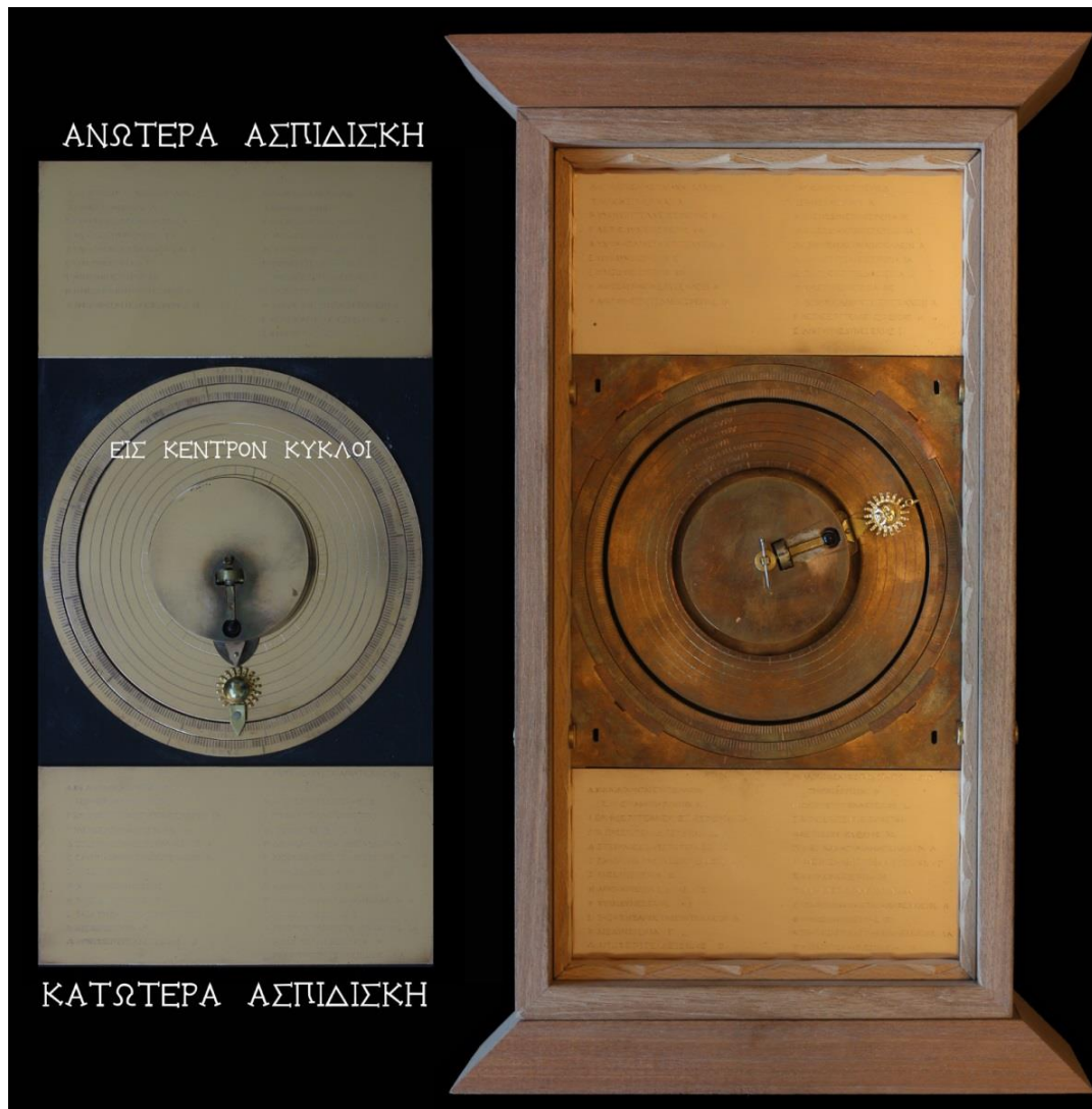
Fig. 15. Left, assembling the parts which are Defined/Described/Referred on the BCI Part-1 text. Right, one of the Antikythera Mechanism functional models designed/constructed by authors (after the final assembling of the parts presented on BCI Part-1). The oxidized central front area was deliberately not polished. Parts constructed in bronze material (94%Cu, 6%Tin). The wooden design of this model is a design view of the first Author. Images by the Authors
