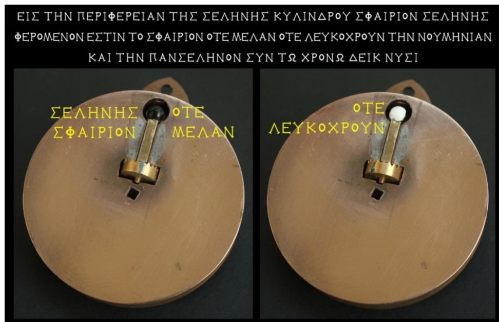
Fig. 6. The Lunar phases sphere which is half white/half blackened. Black and white color alternate during the time of rotation of the small crown gear. Bronze Lunar Cylinder constructed by the authors
