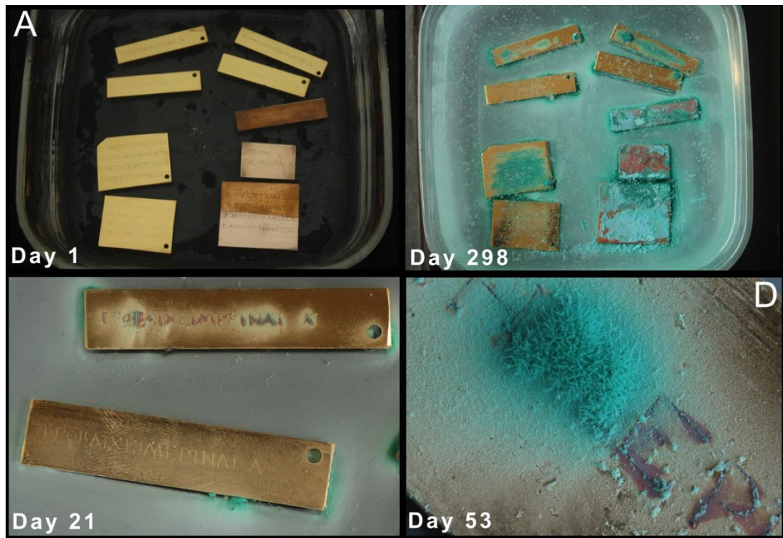
Fig. 2. A) Three pairs of gilded bronze pieces (two pairs on top and one on bottom left) were used for the following corrosion experiment: One piece of each pair was firstly gilded and afterwards engraved (therefore, each engraved letter is not gilded). The second piece was firstly engraved and then was gilded. Afterwards, the pieces were immersed in a solution of sea water with salinity of about 38.5, close to that of the Antikythera sea water, using raw sea salt from Kythera. The three pieces on bottom right are (totally) non-gilded bronze. B) After 298 days, each piece exhibits a different corrosion level. Visible products of bronze corrosion by sea water are: copper chlorides in turquoise shades, copper oxides in dark red/brown shades. 19 C, D) After about 2-3 weeks, non-gilded letters begin to show corrosion signs and as times passes, the corrosion increases the letter depth (for the chemical procedure see Voulgaris et al., 2019b). On the other hand, totally gilded pieces don't show any corrosion signs, since gold is highly resistant to sea water corrosion. 20 Since the Mechanism's bronze material is prone to short term oxidization, the manufacturer could have gilded them before the engraving. C) The corrosion of the simple bronze engraved piece is evident. D) The concentration of crystal copper chlorides is visible. Material process and corrosion experiment by the Authors. The images were taken after the use of an optomechanical system with several focal lengths, in macro, with micro x-y movements and differential mechanical micro focus, designed/constructed/used by the first Author
