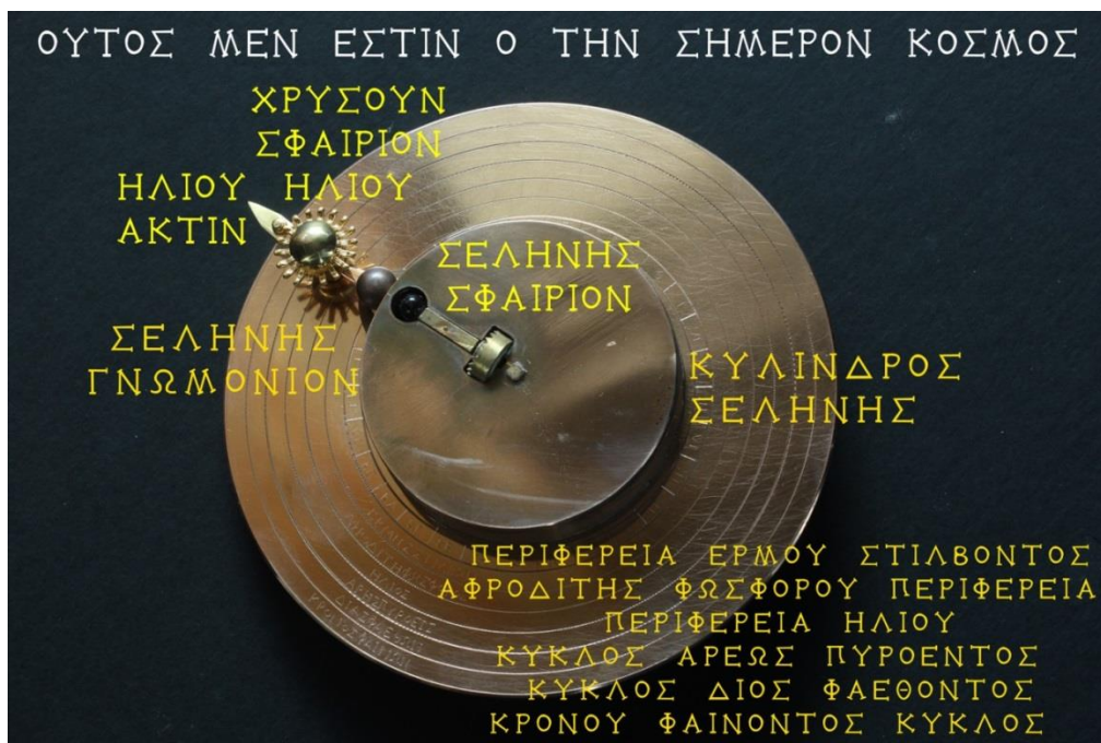
Fig. 12. The Presentation of the Hellenistic ΚΟΣΜΟΣ (Cosmos) of the Antikythera Mechanism: The Earth is located in the geometrical center, the Lunar Disc/Cylinder, the Lunar Phases Sphere, the orbits of the inferior planets, the Golden Sphere with the Solar Ray-pointer and the orbits of the superior planets. Material and image by the Authors
