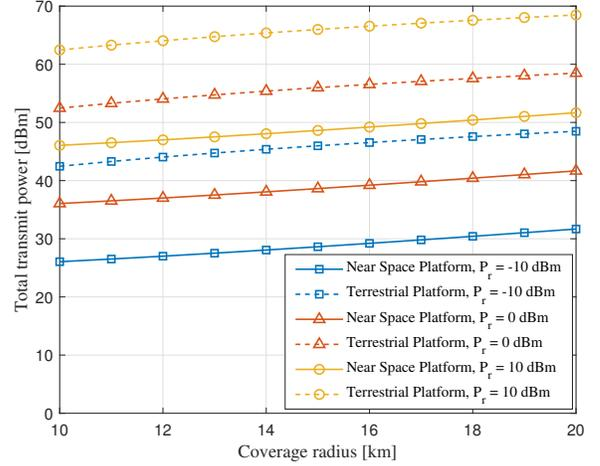
Fig. 4. Comparison of power consumptions between NS-COM and the classical terrestrial cellular networks with respect to the coverage radius, under different values of received power at the cell edge user.
