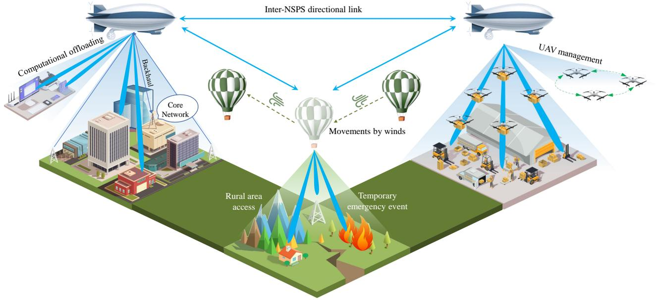
Fig. 5. Illustrations of the near-space access network and mesh network, where different applications of the near-space access network are presented, including Internet access for distant and disaster regions, dual-hop wireless backhauling, offloading of data traffic or computational tasks and management for UAV fleet and cargo drones.
