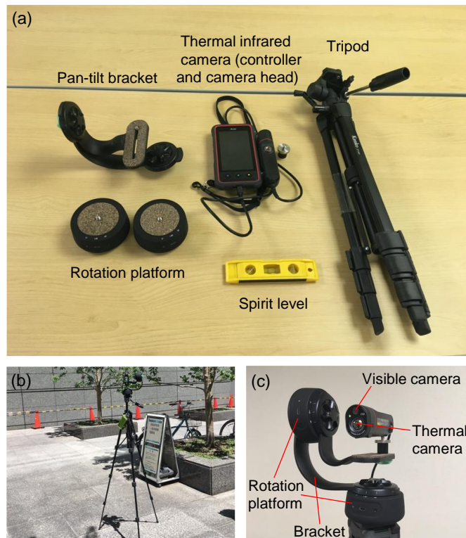
Fig. 1. Photographs of the developed system: (a) instruments comprising the system; (b) appearance of the system; (c) magnified view of camera part.
