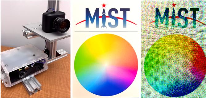
Fig. 2. Left: The experimental setup with a DLP LightCrafter 4500 Evaluation Module and a Prophesee evaluation kit (Gen3-VGA). Middle: Printed color wheel with the logo of the MIST Lab., captured by a frame-based high-resolution camera. Right: Colorful image reconstructed by proposed method captured by monochrome EC aided by SL.
