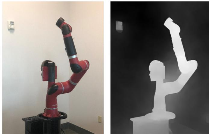
**Figure 2. Top row is RGB and Depth images taken on iPhone X camera**
